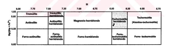
Figure 63. Plots of amphibole samples on the Si and Mg/(Mg+Fe<sup>2+</sup>) diagram for (Ca+Na)<sub>B</sub> $\geq$ 1.34, Na<sub>B</sub><0.67, (Na+K)<0.50 and Ti<0.50 (After Leake, 1978).
