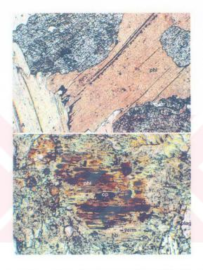
Figure 32. Photomicrographs showing oxide inclusion within phlogopite. A: (PPL, x10), B: (PPL, x10) (phl: phlogopite, py: pyroxene, hb: hornblende, plagioclase:plagioclase, verm: vermiculite, op: opaque).
