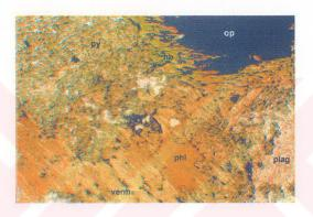
Figure 24. Photomicrograph showing actinolitic hornblende development (PPL, x2.5) (py: pyroxene, hb: hornblende, phl: phlogopite, plag: plagioclase, verm: vermiculite).
