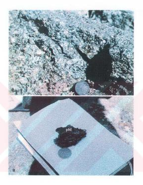
Figure 14. Phlogopite gabbro containing small amount of pyroxene and plagioclase (A) outcrop of phlogopite gabbro, (B) hand specimen of phlogopite gabbro (phl: phlogopite, py: pyroxene, plag: plagioclase).
