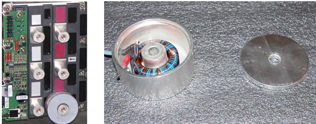
Figure 3.67 CT1 and CT2 Current Transformers
