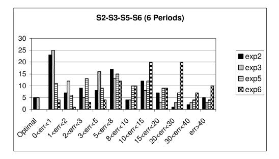
Figure A.11 Error distributions of Non-myopic algorithm for sample sets S2, S3, S5 and S6 for 6periods planning horizon.
