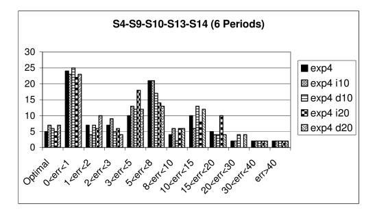
Figure A.35 Error distributions of Non-myopic algorithm for sample sets S4, S9, S10, S13 and S14 for 6 periods planning horizon.
