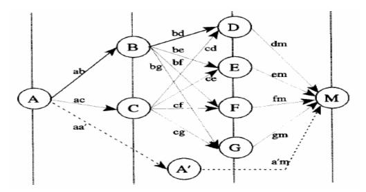
Figure 2.2 A disassembly process represented by a graph, Penev and De Ron (1996)
