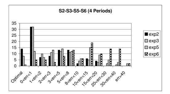
Figure A.4 Error distributions of Non-myopic NC-first algorithm for sample sets S2, S3, S5 and S6 for 4 periods planning horizon.
