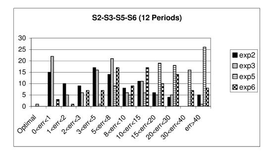
Figure A.9 Error distributions of Myopic algorithm for sample sets S2, S3, S5 and S6 for 12 periods planning horizon.
