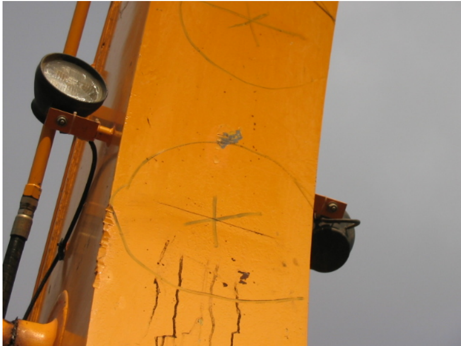
Figure 3.5 Flaw in excavator structure
