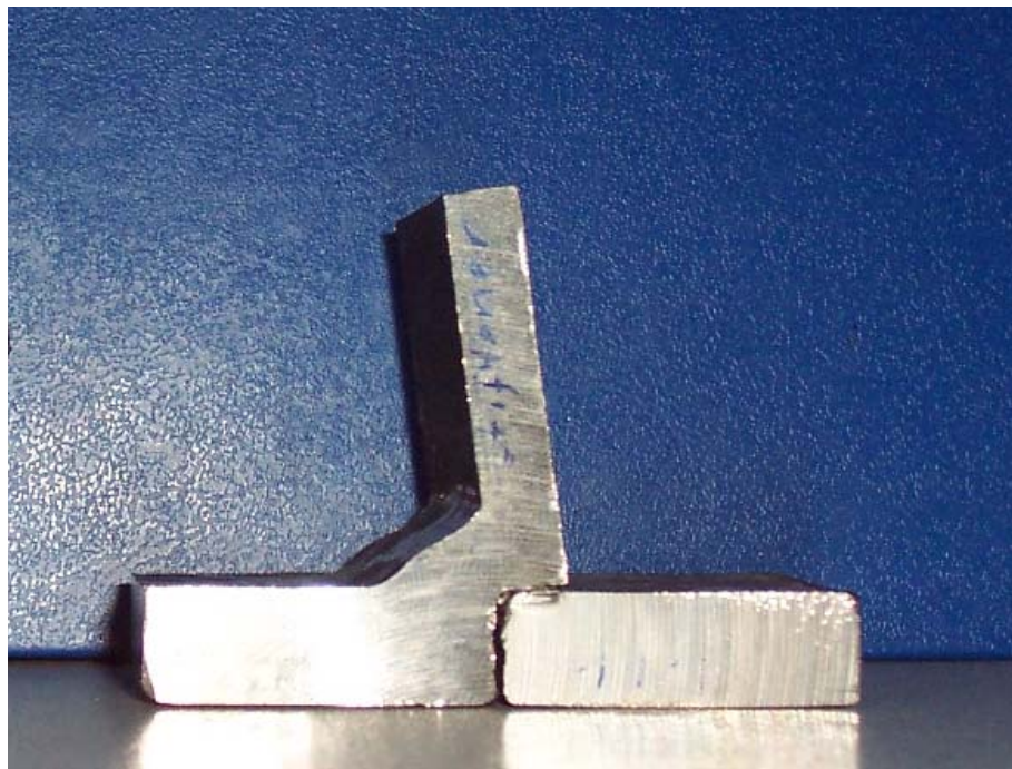
Figure 3.7 Crack propagation due to weld gap
