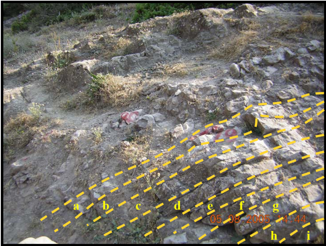
Figure 28: Field photograph of impure limestone (a: grey shale, b: limestone, c: limestone, d: black shale, e: limestone, f: siltstone, g: grey shale, h: limestone, i: conglomerate).
