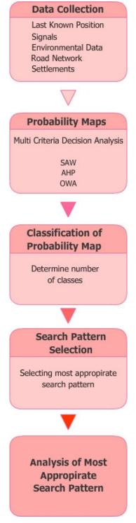
Figure 3-1 Stages of Developed Methodology
