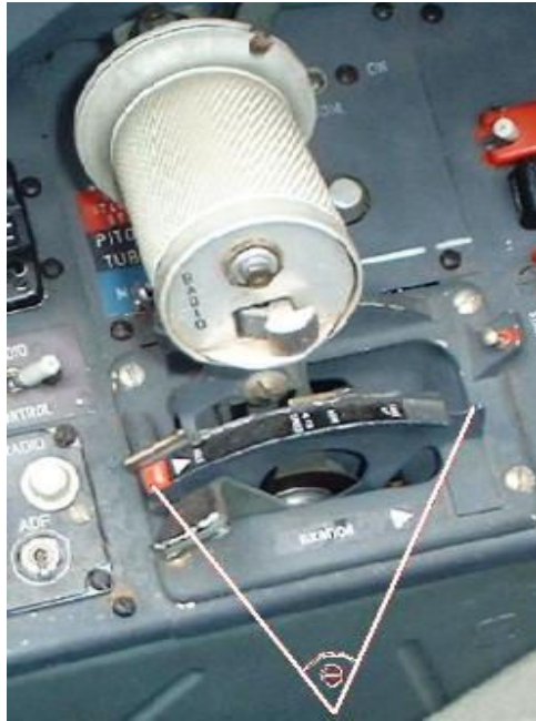
Figure 4.18 Throttle Lever Setting Rang in L-39 Left Side Panel.
