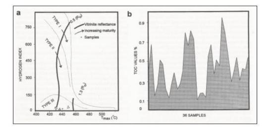
Figure 5.13: a) Rock-Eval Pyrolisis and b) Total Organic Carbon (TOC) Analyses of the Shales of the Kusuri Formation from the Sinop Region [21]
