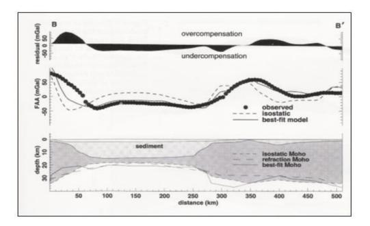
Figure 5.4: Gravity and state of flexure in the Western Black Sea (Detail of BB' Section in **Figures 5.1 & 5.2**) [20]
