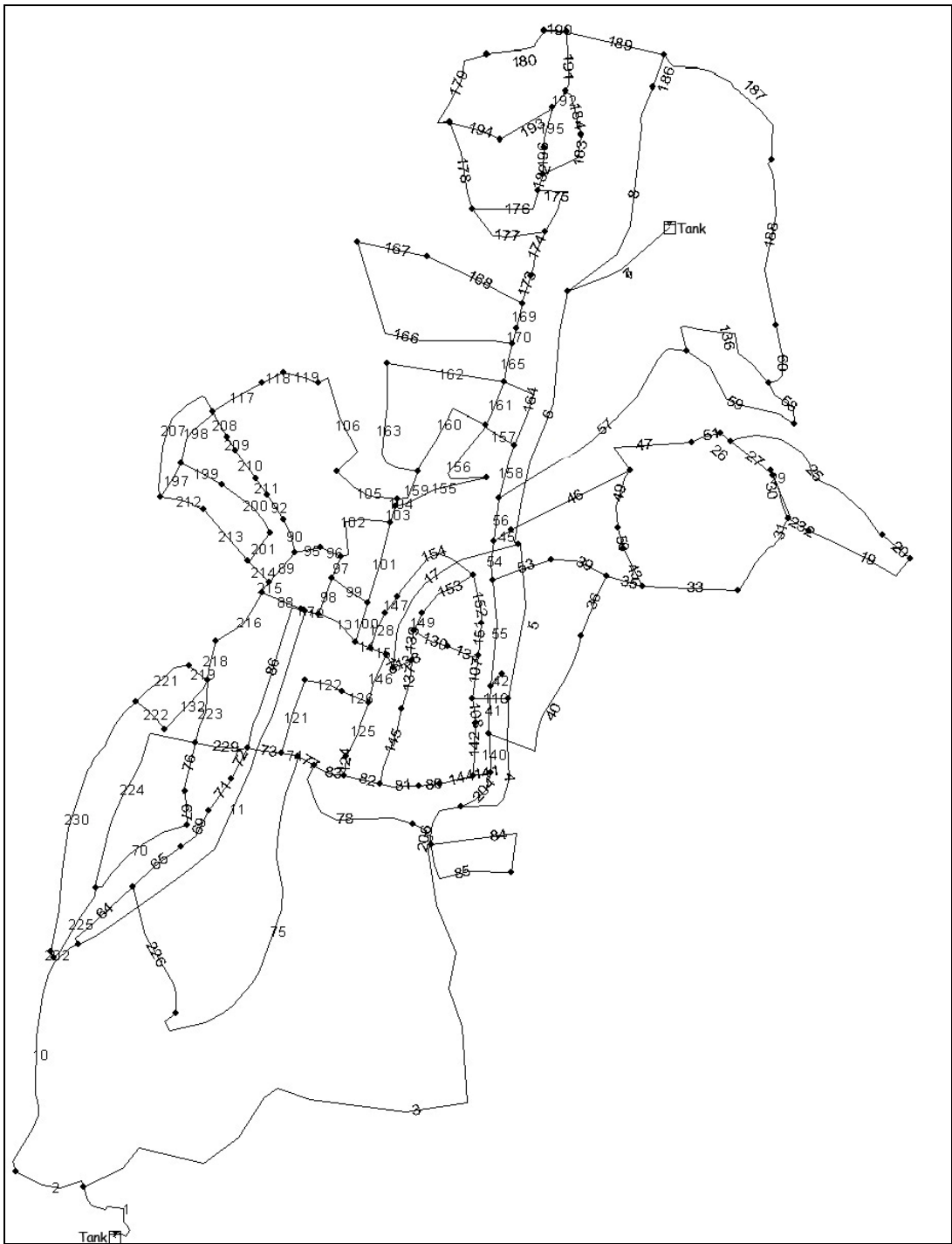
Figure 6.2. Layout of N8-1 Network with Pipe IDs
