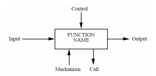
Figure 2.6. Arrow positions and roles in IDEF0 Diagram
