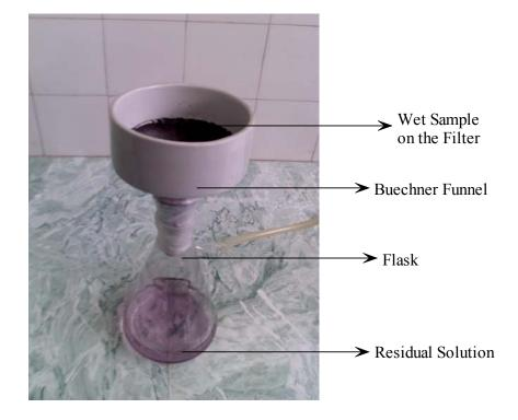
Fig.3.10 Experimental set-up of filtration and obtained sample and residual solution
