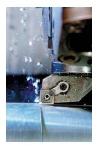
Fig.2.2 Metal tip coated with TiB<sub>2</sub> while machining aluminum alloy [36]
