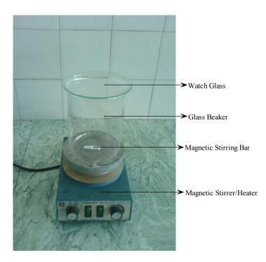
Fig.3.9 Experimental set-up of leaching without heating
