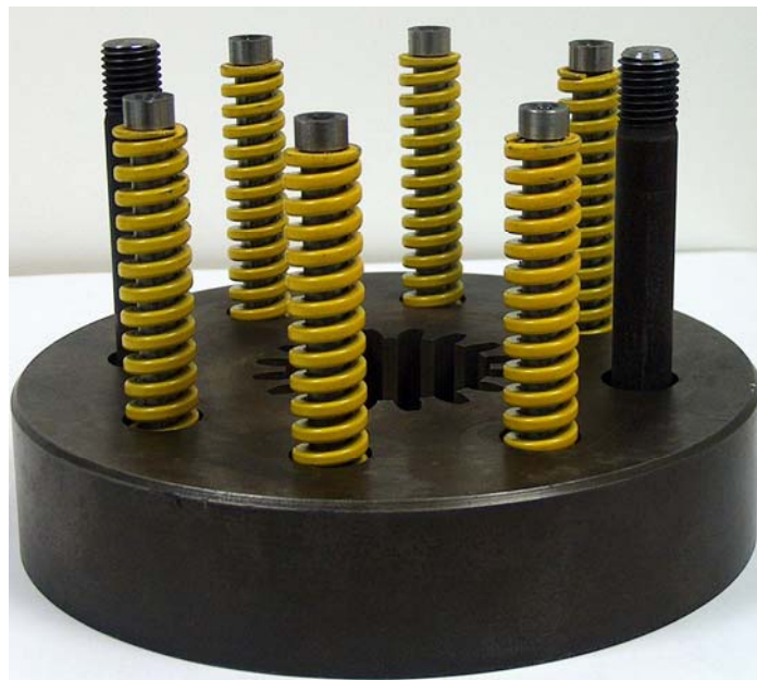
Fig.5.23 A view of Middle Die with Helical Springs and Restriction Bolts Attached
