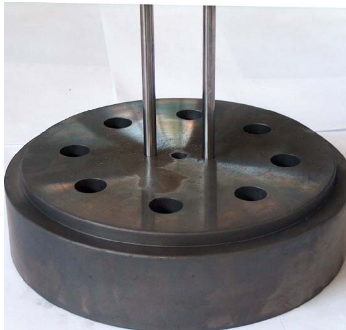
Fig. 5.18 A view of Base Section of Lower Die and Ejectors
