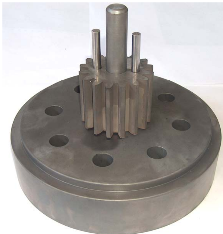
Fig.5.20 A view of Manufactured Lower Die Assembly
