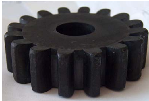
Fig.6.10 Front View of the Formed Gear
