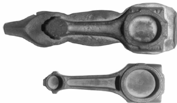
Fig.2.2. Conventionally forged and precision forged connecting rod [15]
