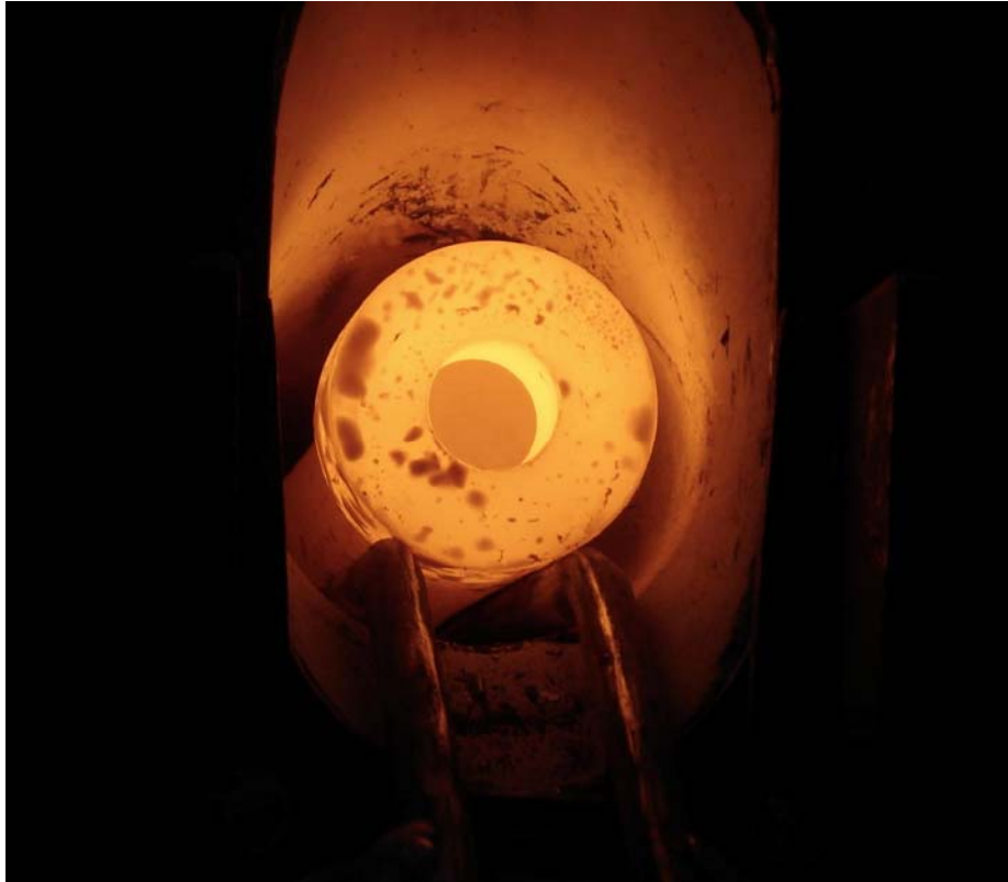
Fig.6.5 A view of Heated Tube Shaped Billet inside the Heater
