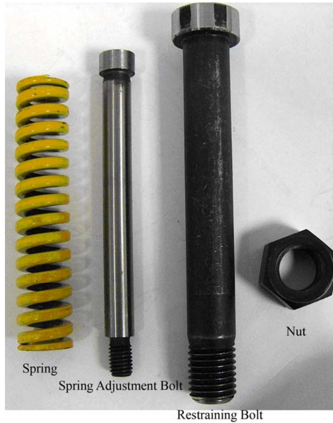
Fig.5.22 Spring, Spring Adjustment Bolt, Restraining Bolt, Nut
