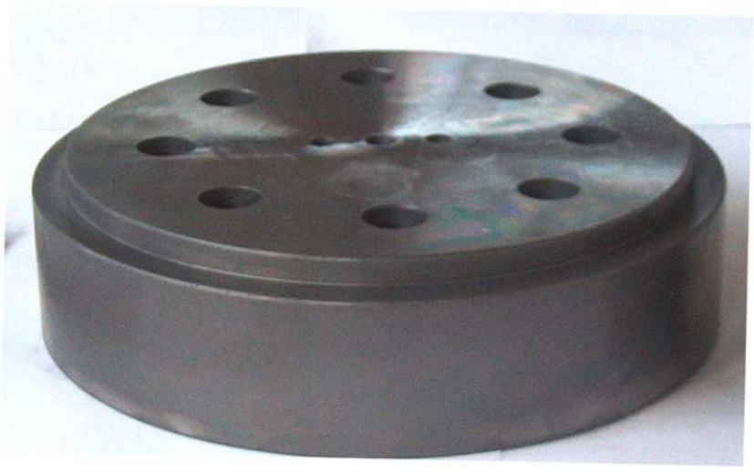
Fig.5.9 A view of Manufactured Base Section of the Lower Die
