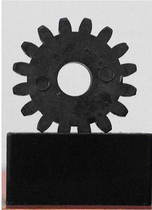
Fig.6.9 A view of Formed Gear
