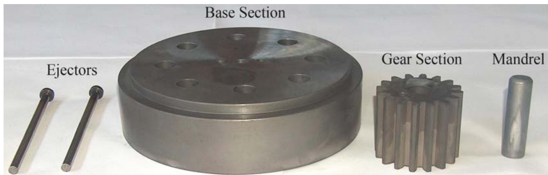
Fig.5.15. A view of Lower Die Assembly
