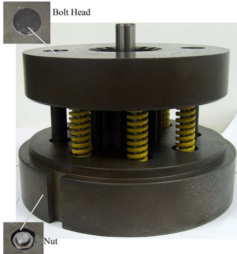
Fig.5.24 A view of Middle Die and Lower Die
