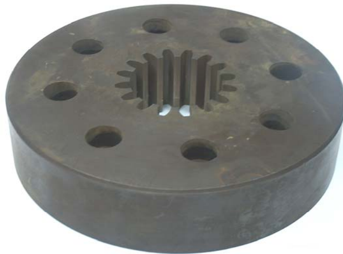
Fig.5.13 A view of Manufactured Middle Die
