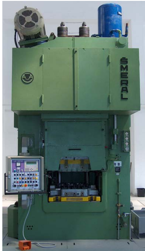
Fig.5.1 A view of Smeral 1000-ton Mechanical Press in METU-BILTIR Center Forging Research and Application Laboratory
