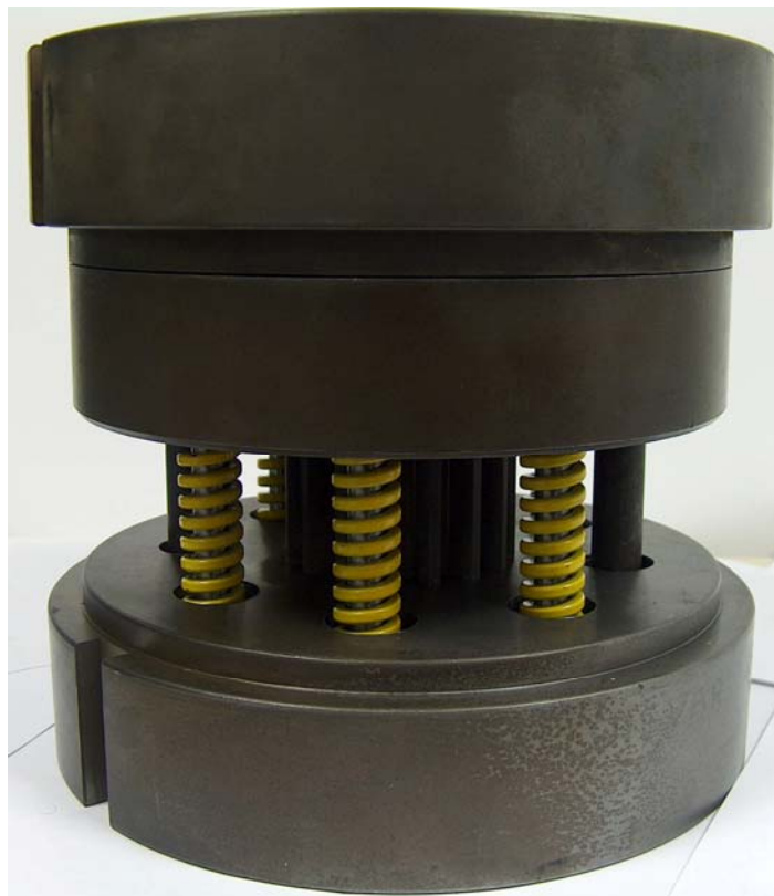
Fig.5.25 A view of Complete Assembly of the Precision Forging Die Set
