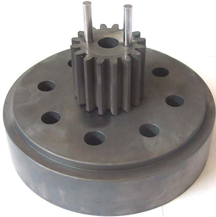
Fig.5.19 A view of Base Section of Lower Die, Ejectors and Gear Section
