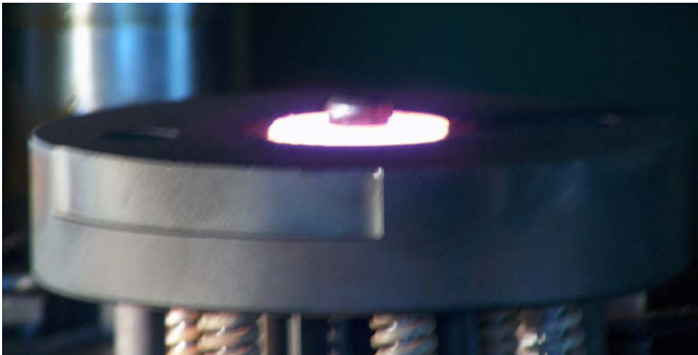
Fig.6.6 A view of Heated Tube Shaped Billet inside the Middle Die
