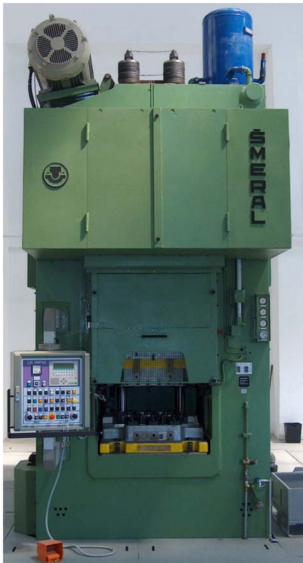
Fig.D.1. Smeral 1000 ton mechanical press in METU-BILTIR Center Forging Research and Application Laboratory
