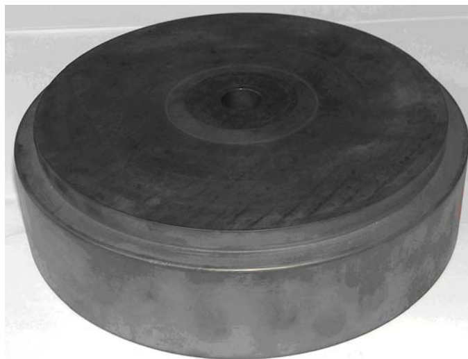
Fig.5.7. A view of Manufactured Upper Die
