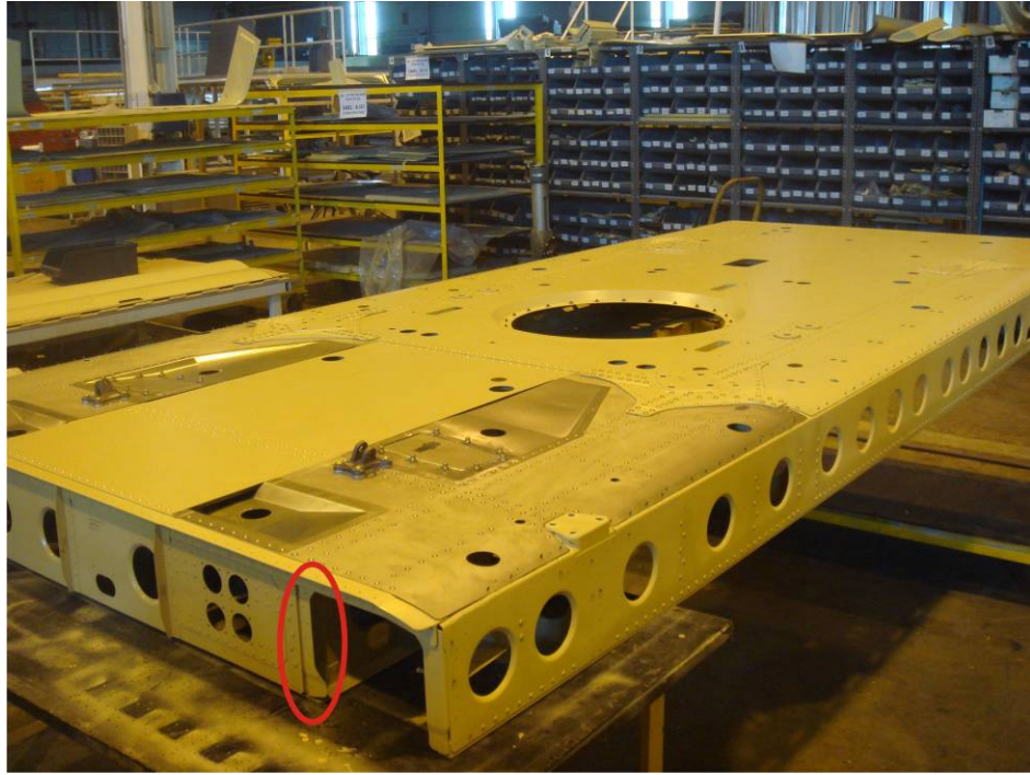
Figure 6.1 The location of the part case 1 in the upper shell of Agusta AB-139 aircraft.
