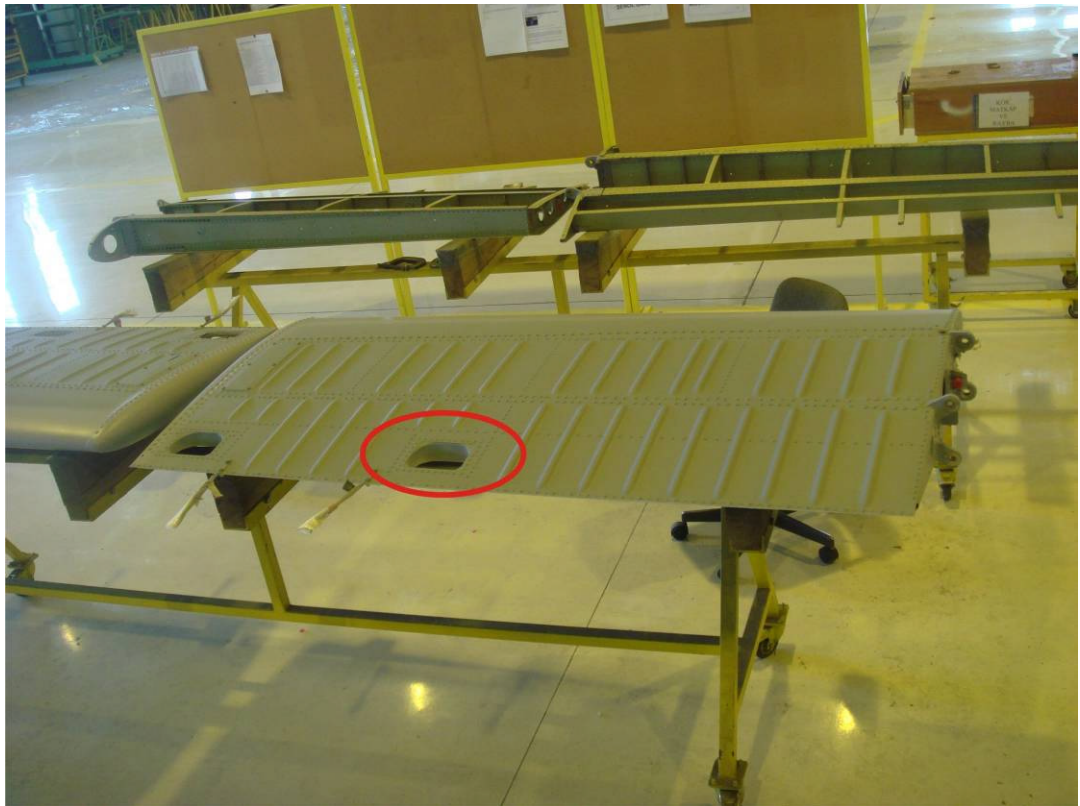
Figure 6.9 The location of the part case 3 in the horizontal stabilizer of Sikorsky UH-60 helicopter
