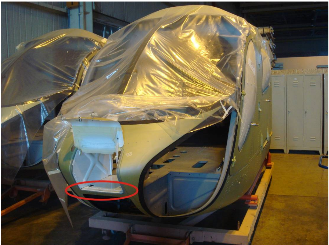
Figure 6.5 The location of the part case 2 in the cockpit of McDonnell Douglas 902 helicopter
