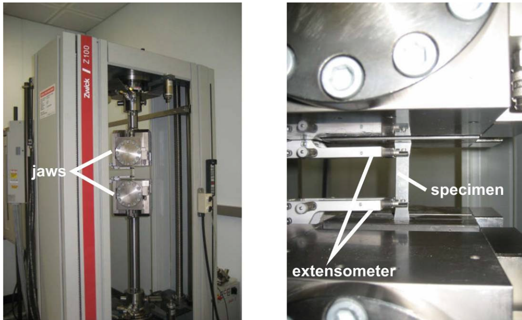
Figure 4.10 Uniaxial tensile testing of Aluminum sheet.
