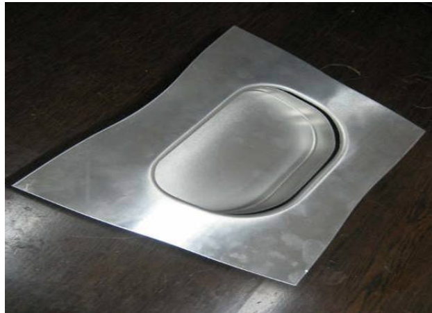
Figure 6.10 Split part after forming in the flexform press.
