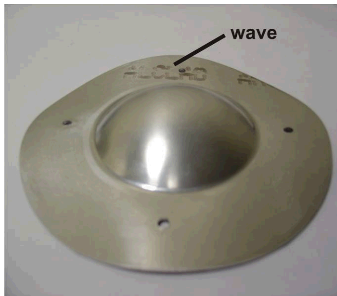
Figure 4.9 Wavy view of the circular bulging specimen.
