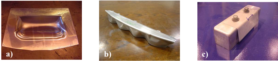
Figure 1.3 Failure modes of the process: a) tearing b) wrinkling c) springback
