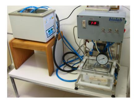
Figure 2.2. Custom-made pressure chamber
