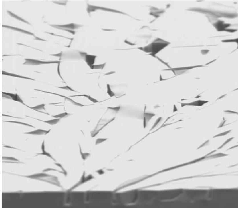
Figure 2.4: SEM image of a masking resist cracked at cryogenic temperature during the etch process [31].
