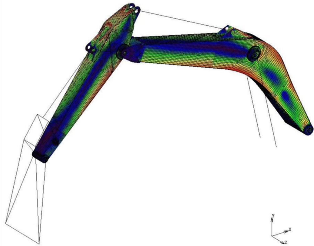
Figure 4.4 Von Mises Stress Map for Shell Outer Layer
