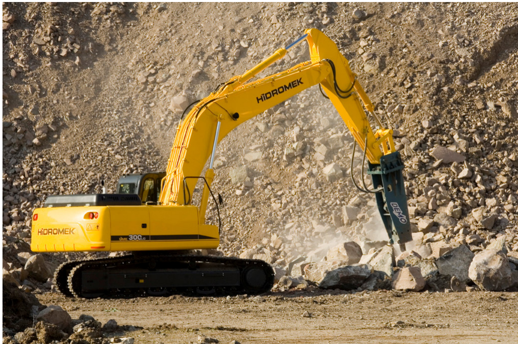
Figure1.3: An example for excavator used by changing the attachment only (Breaker)
