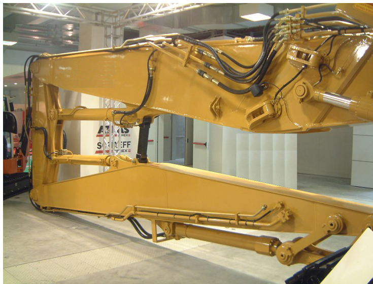
Figure 3.10: An example for demolition excavator transportation position
