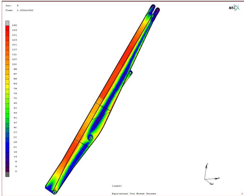
Figure 5.11: View-1 of the boom of the final design results
