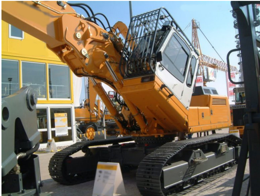
Figure 6.4: An example for the cabin of a demolition excavator
