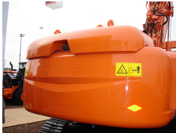
Figure 6.3: An example for the additional counterweight of a demolition excavator
