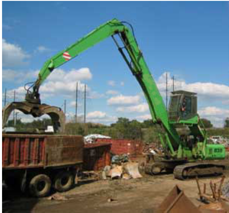
Figure1.4 An example for excavator designed by changing the attachment and the booms for long reach (Material Handler)
