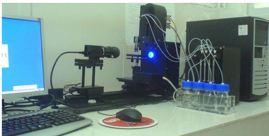
Figure 2.3 Goniometer used in contact angle measurements
