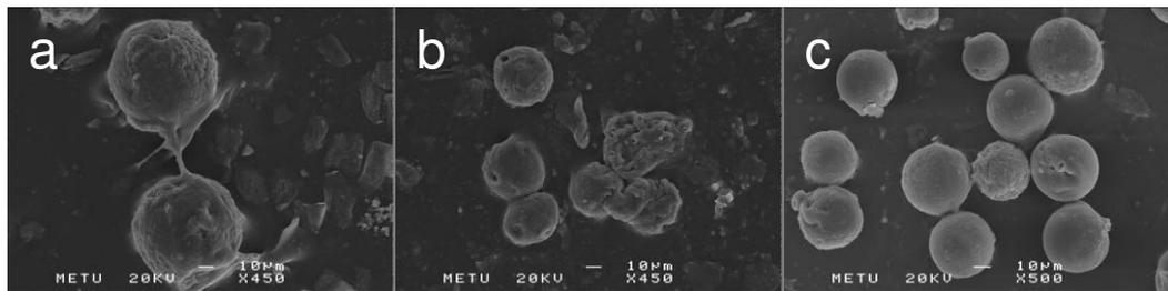
Figure 3.1 SEM results of chitosan microspheres prepared with different amounts of GA (a) CH-1.25, (b) CH-2.5 and (c) CH-5.0
