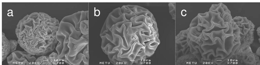
Figure 3.3 SEM pictures of semi-IPN microspheres (a) CH:PVP-1:1, (b) CH:PVP-1:0,5 and (c) CH:PVP-1:0,33
