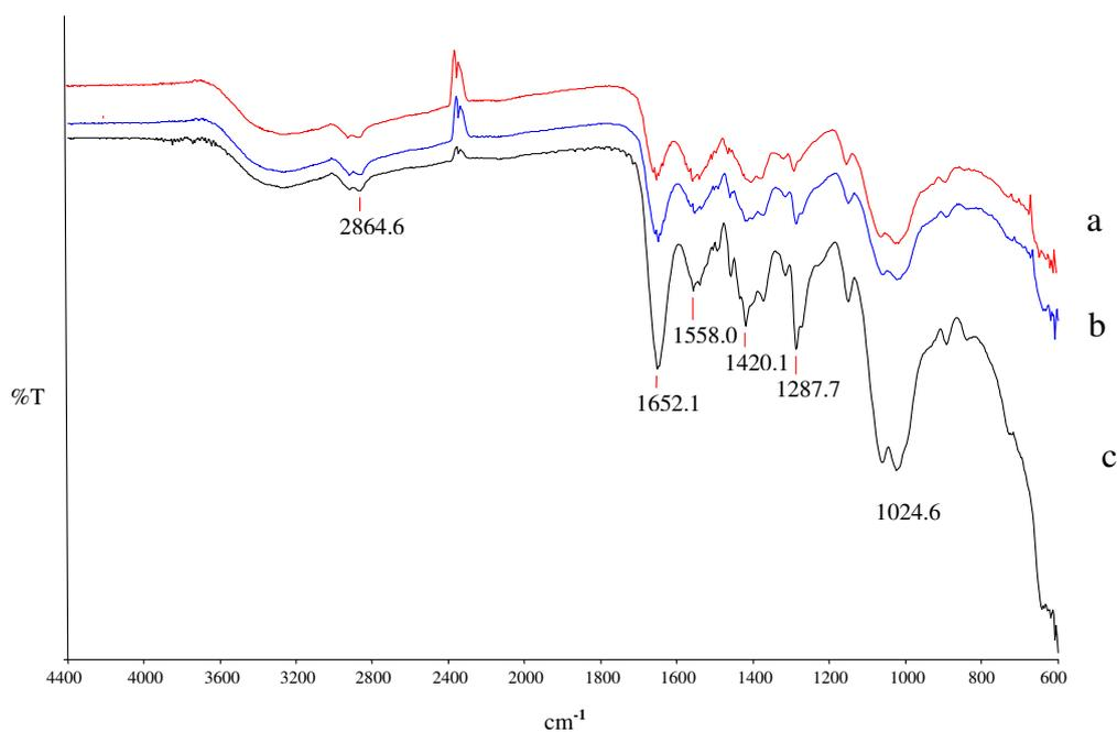
Figure 3.5 ATR spectra of films (a) CH:PVP-1:1-5, (b) CH:PVP-1:0,5-5 and (c) CH:PVP-1:0,33-5
