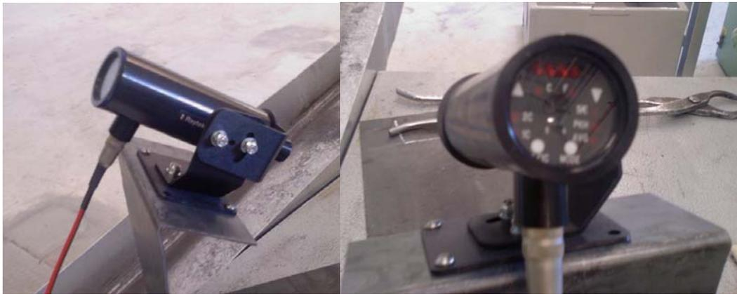
Figure 4.10 Raytek marathon series MR1SASF model optical pyrometer
