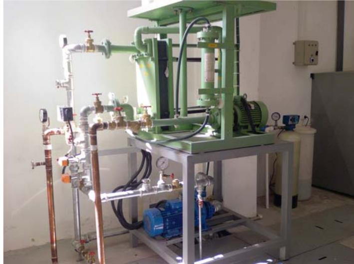
Figure 4.3 Heat Exchanger of the Cooling Unit
