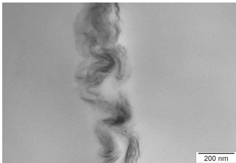
Figure 4.1.22. TEM micrograph of PP/2 wt% Cloisite® 25A/5 wt% Lotader® 8900 E-MA-GMA nanocomposite processed by (PE)C2 mixing sequence.
