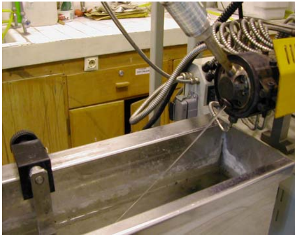
Figure 3.2.1.b. The die and control panel of Thermo Prism TSE 16.
