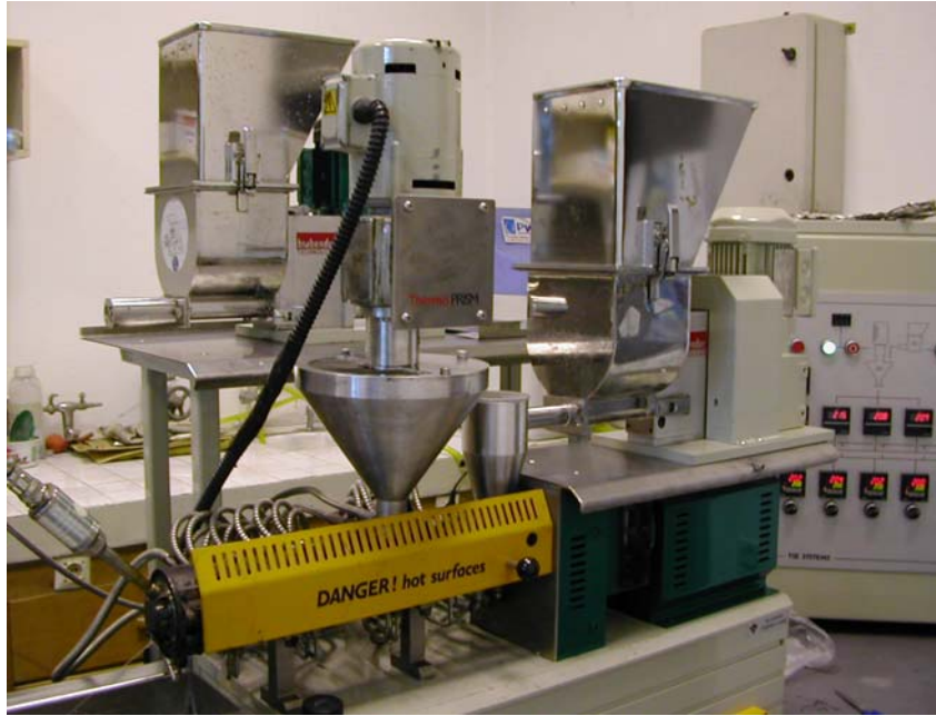
Figure 3.2.1.a. Thermo Prism TSE 16 co-rotating twin screw extruder.
