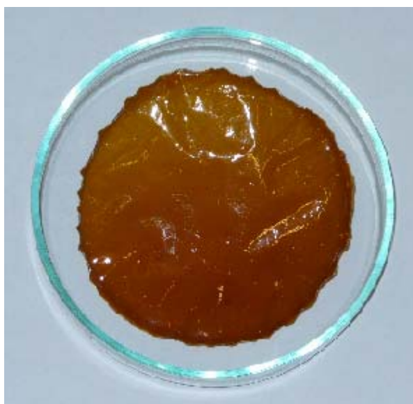
Figure 11. A picture of an acid doped mPBI membrane prepared
