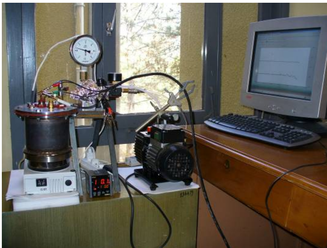
Figure 15. A picture of the complete setup used for the conductivity measurements
