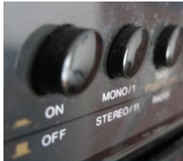
Figure 2-13 Latching Push Buttons
