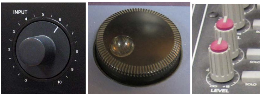
Figure 2-24: Left: Rotary Knob, Center: Rotary Knob recessed to ease controlling, Right: Rotary Knob with Pointer.
