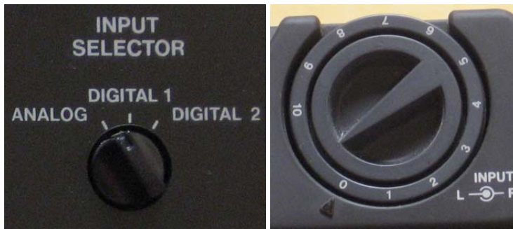
Figure 2-19: Left: Three-Position Rotary Selector, Right: Ten-position Rotary Selector.
