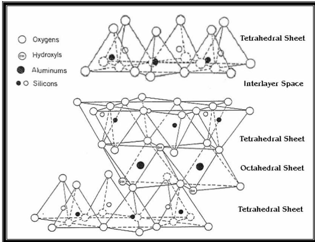
**Figure 3. Schematic representation of the crystal structure of a 2:1 type clay mineral showing the relations between tetrahedral and octahedral sheets and interlayer spaces (Clauer and Chaudhuri, 1995).**
