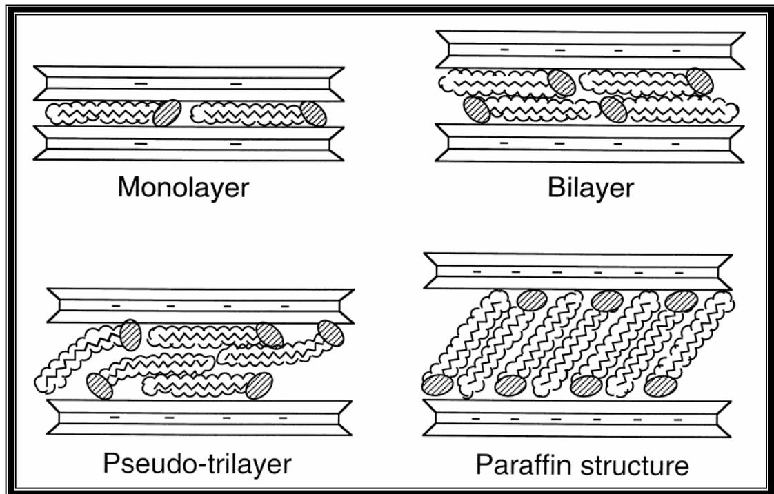
**Figure 4. Orientation of alkylammonium ions in the galleries of layered silicates with different layer charge densities (Lagaly, 1986).**
