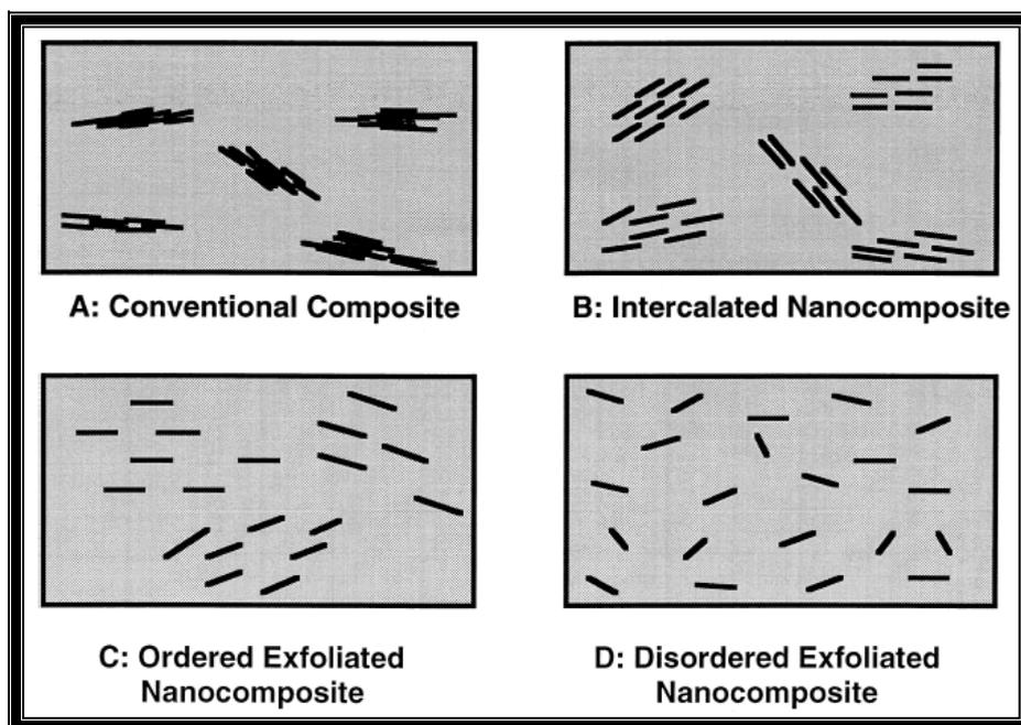
**Figure 6.** Schematic illustrations of (A) a conventional; (B) an intercalated; (C) an ordered exfoliated; and (D) a disordered exfoliated polymer–clay nanocomposite (Le Baron et al., 1999).
