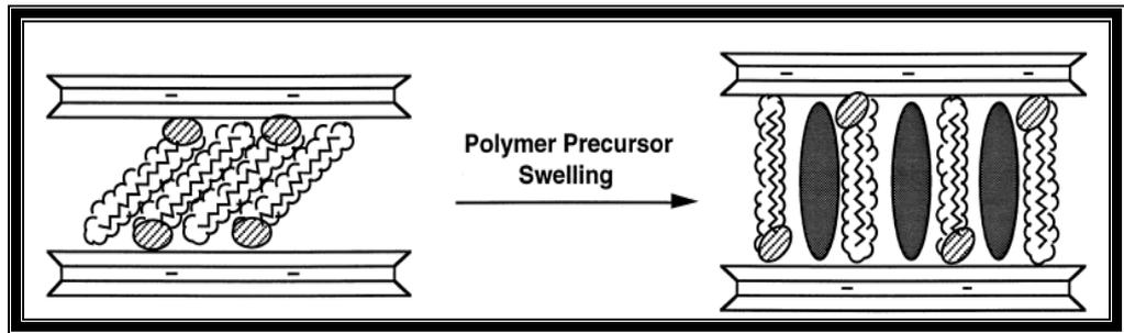
**Figure 7.** Proposed model for the swelling of alkylammonium exchanged clay with a parafin structure by polymer precursors (Le Baron et al., 1999).
