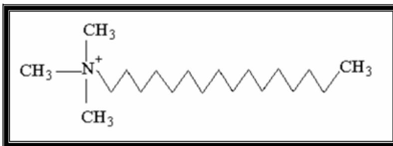
Figure 15. Hexadecyltrimethylammonium ion ( $R=C_{16}H_{33}$ ) (Inam, 2006).
