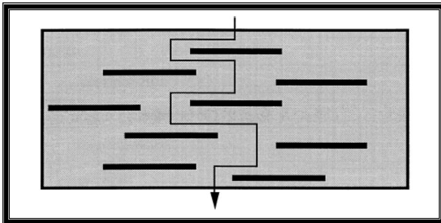
**Figure 8.** Proposed model for the tortuous zigzag diffusion path in an exfoliated polymer–clay nanocomposite when used as a gas barrier (Yano et al., 1993).
