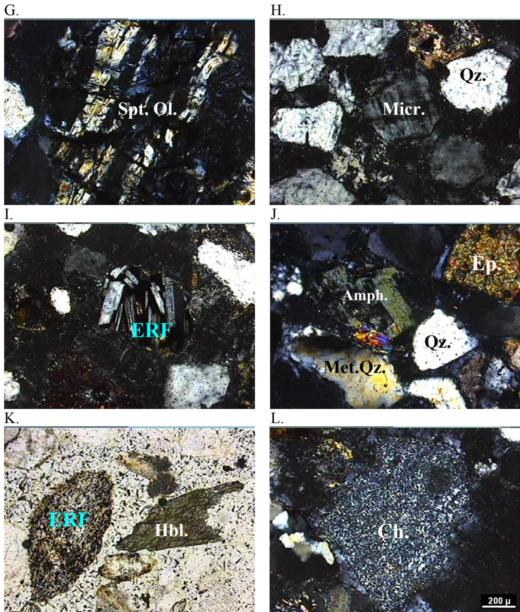
Figure 12 (continued). Thin sections (XPL except for K, which photo was taken using PPL) of sand sample used in permeability test (Spt.Ol: Serpentinized Olivine, Micr: Microcline ERF: Extrusive Igneous Rock Fragments, Qz: Quartz, Ep: Epidote, Met.Qz.: Metamorphic Quartz, Amph.: Amphibole, Ch: Chert, Hbl: Hornblende).
