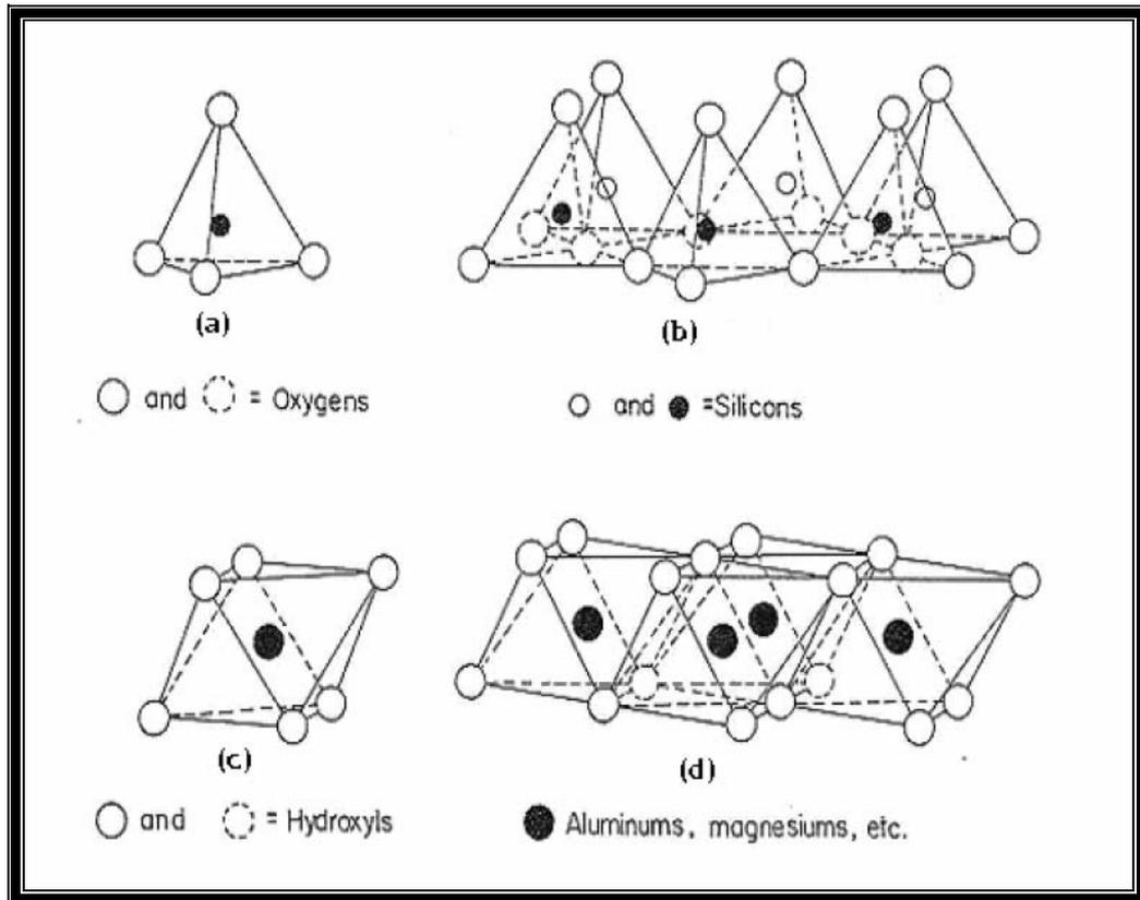
Figure 1. Tetrahedral and octahedral sheet structures in clay minerals (a) single tetrahedral unit, (b) sheet structure of the tetrahedral units, (c) single octahedral unit (d) sheet structure of octahedral units (Grim, 1953)
