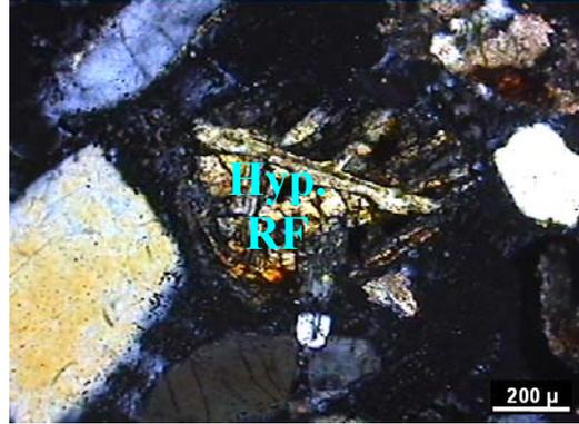
**Figure 12 (continued). Thin sections (XPL except for K, which photo was taken using PPL) of sand sample used in permeability test. (Cc: Calcite, Hyp. RF: Hypabyssal Igneous Rock Fragments).**
