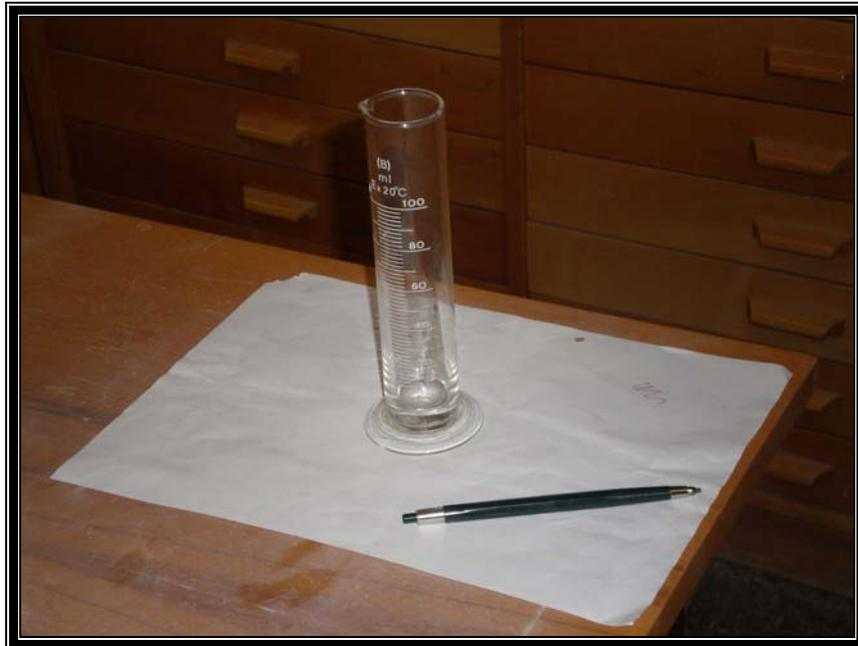
Figure B1. Apparatus for determination of swelling capacity
