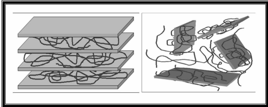
**Figure 5.** Schematic illustration of two different types of thermodynamically achievable polymer/clay nanocomposites. Left: the intercalated system, where the polymer chains penetrate into and swell the galleries of the silicate layers. Right: the exfoliated or delaminated system, where individual silicate layers are dispersed in the polymer matrix (Dulgerbaki, 2006).
