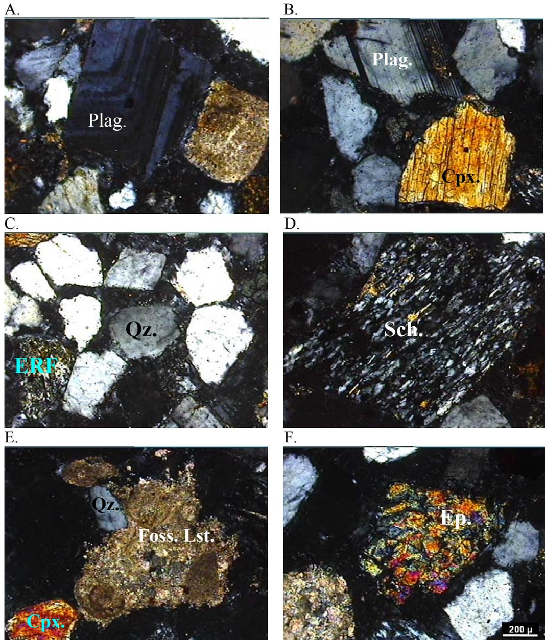
**Figure 12.** Thin sections (XPL) of sand sample used in permeability test (Plag.: Plagioclase, Cpx: Clinopyroxene, ERF: Extrusive Igneous Rock Fragments, Qz: Quartz, Sch: Schist, Foss. Lst: Fossiliferous Limestone, Ep: Epidote).
