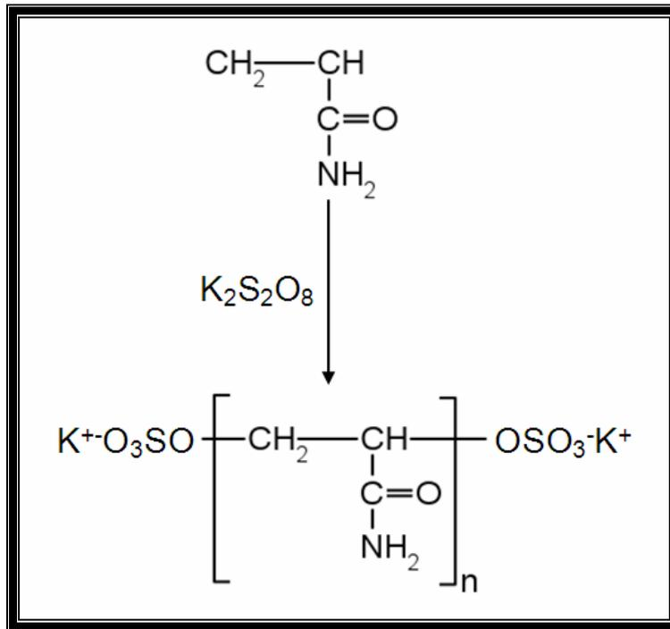
**Figure 17. General radical reaction of polyacrylamide with  $\text{K}_2\text{S}_2\text{O}_8$**
