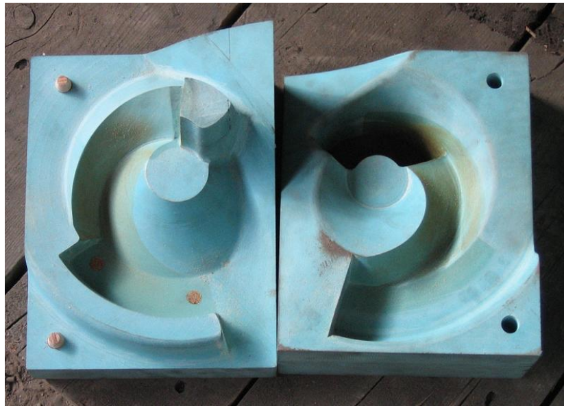
Figure A.1 Core box of impeller
