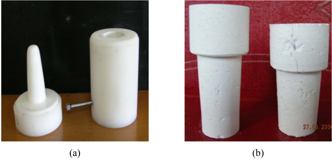
Figure 3.1 (a) Polyamide moulds used in alumina crucible production. (b) Two crucibles with the one on the left hand side was prepared by the polyamide mould free of surface cracks and the one on the right hand side produced by conventional technique containing cracks.
