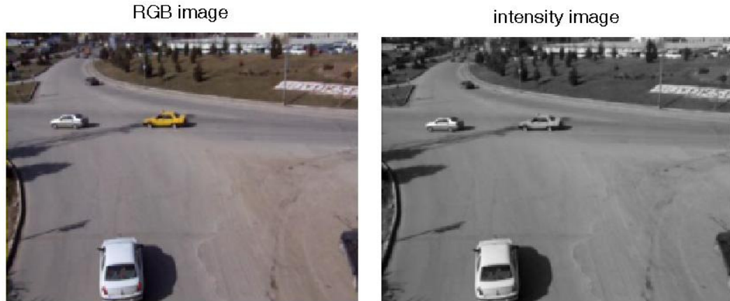
Figure 2-1: RGB Image and Grayscale (Intensity) Image
