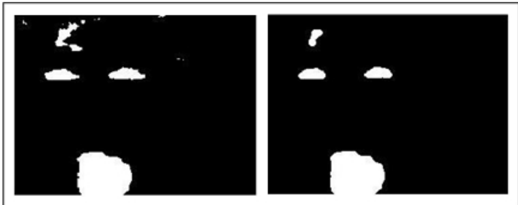
Figure 2-7: Morphologic Operators – Opening Process Example
