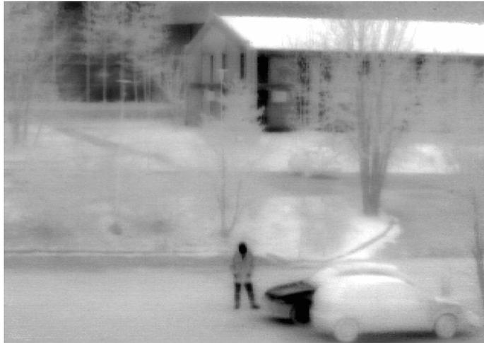
Figure 7.17 Windowed 640x448 image of InP/InGaAs QWIP at 70K with 7.5 ms integration time using 50 mm effective focal length lens [96].
