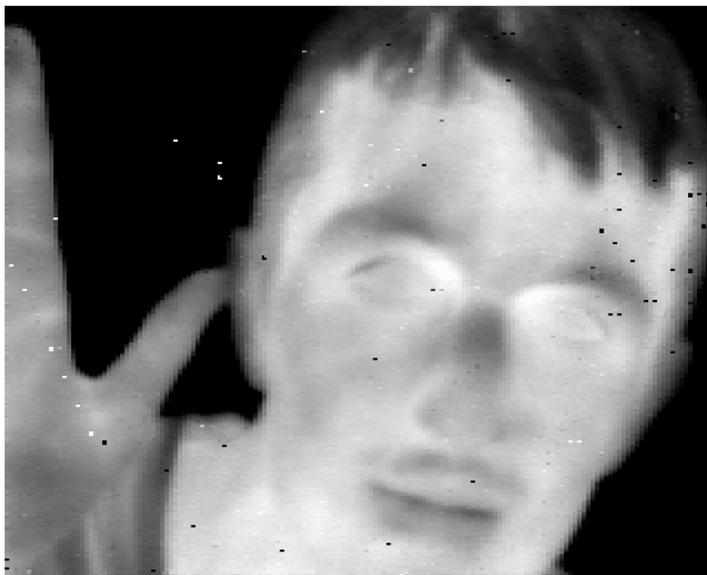
Figure 7.22 Windowed 320x256 image of InP/InGaAsP QWIP at 70 K using 50 mm effective focal length lens.
