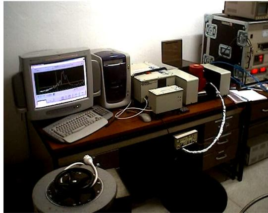
Figure 6.8 Spectral response measurement set-up with FTIR.
