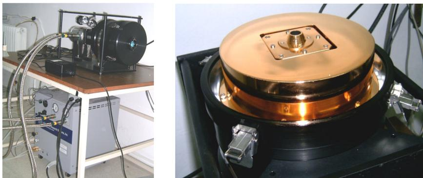
Figure 6.5 Test dewar, He cryostat, and inside of the dewar with f/2 cold shield installed.
