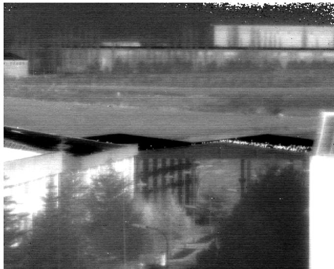
Figure 7.18 Thermal image obtained with 640x512 InP/InGaAs QWIP at 70 K with 17 ms integration time using 150 mm effective focal lens.
