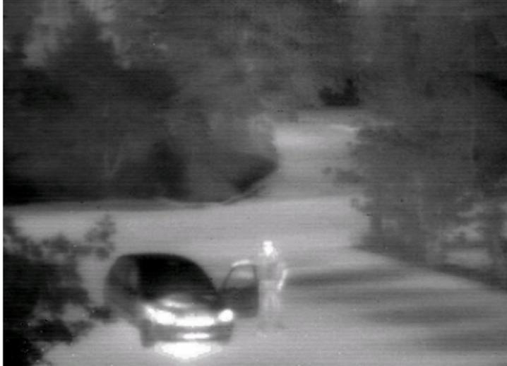
Figure 7.21 Windowed 640x448 image of InP/InGaAs QWIP at 77 K using 50 mm effective focal length lens.
