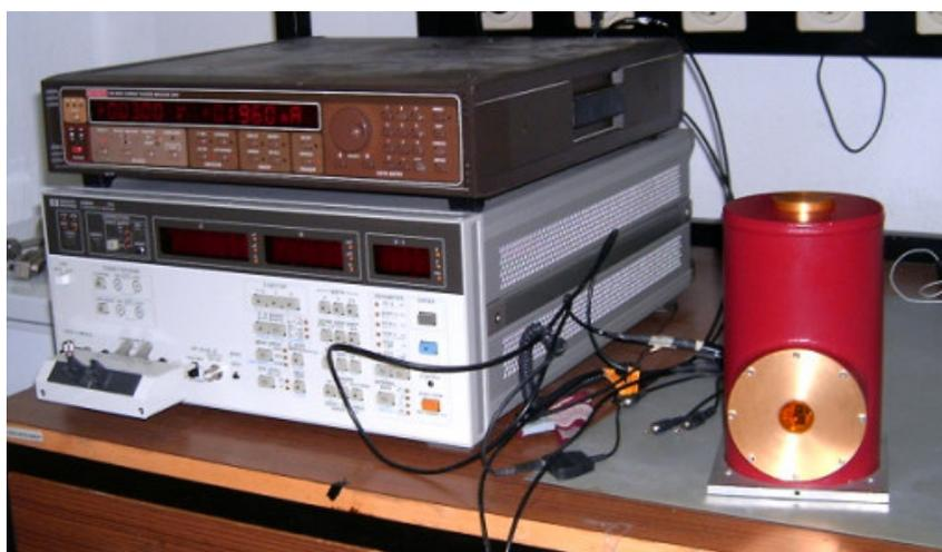
Figure 6.6 I-V Characterization set-up.
