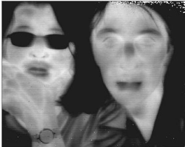
Figure 7.20 640x512 thermal image obtained with InP/InGaAs QWIP at 77 K using 50 mm effective focal length lens [136].
