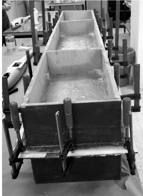
Figure 2.52: Female molds clamped during wing assembly.
