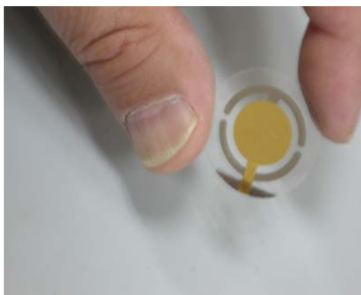
Figure 2.2. 5 MHz quartz crystals (Maxtek Inc., USA) with gold electrodes evaporated on both sides.
