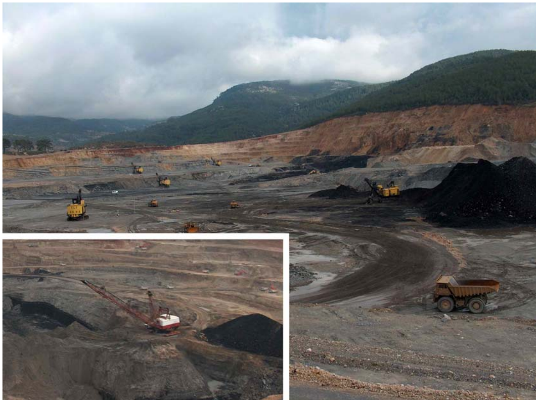
Figure 3.1 General view of open-cast lignite mining site (top: power shovels, bottom:dragline)
