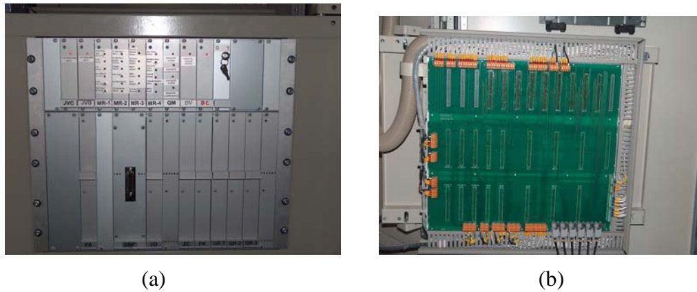
Figure 3.53 Picture of electronic system for CSC based STATCOM (a) front view (b) view of motherboard
