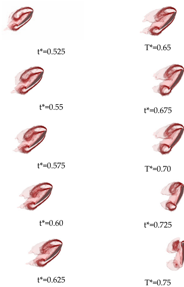
Figure 7.5 (continued) Iso-contours, Q=8 at \alpha=45^\circ , Re = 1000 during the second half upstroke.
