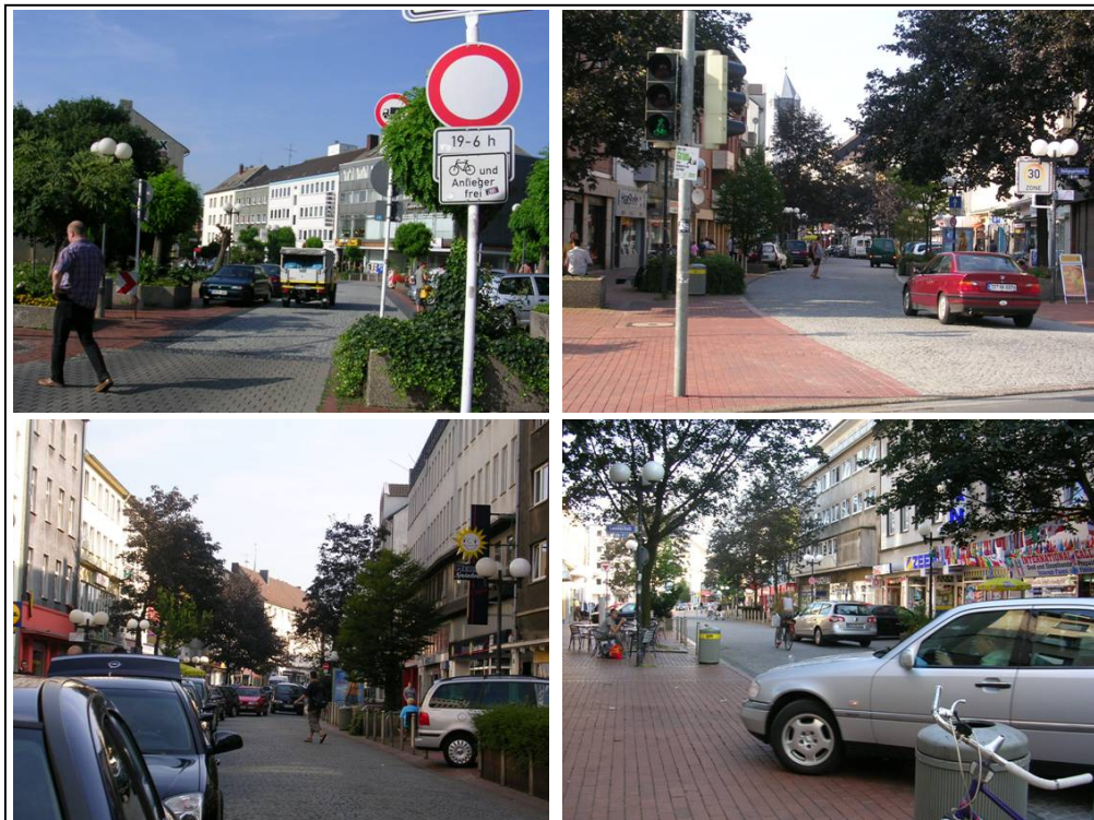
Figure 6.5 Implementation of traffic calming strategies without separation of pedestrian, cyclist, and car traffic in a residential and commercial section of a German city
