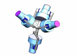
Figure 2.21 Reaction Wheel Configuration
