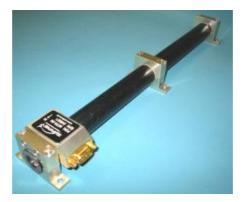
Figure 2.18 MTR 10 Magnetorquer
