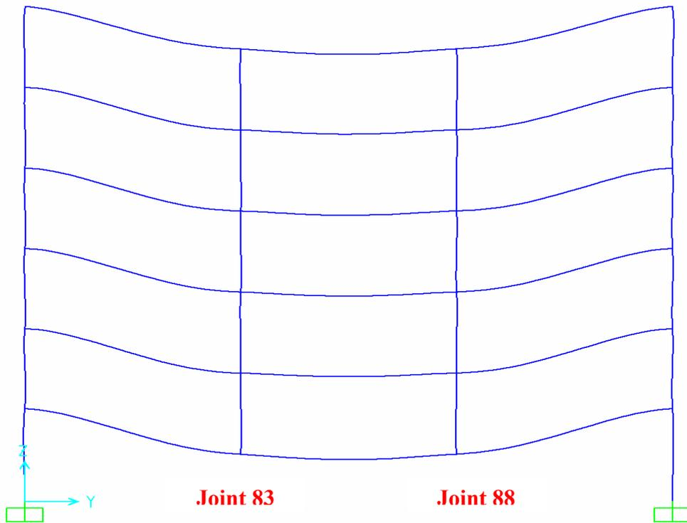
**Figure 46:** Deformed shape of the framing system after two column removal in short direction.
