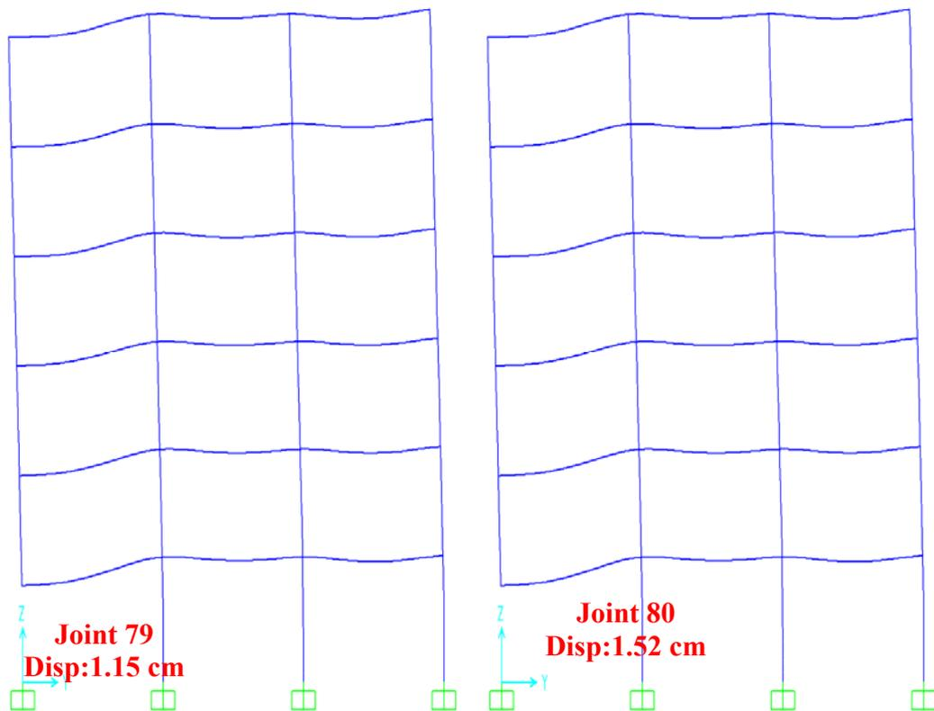
**Figure 43:** Deformed shape and maximum deformation of the framing system after two column removal in long direction. (cross-section of the frame)
