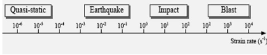
**Figure 7:** Strain rates associated with different types of loading.
