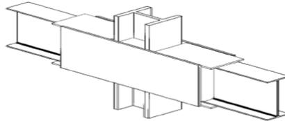
**Figure 32:** SidePlate moment connection system.
