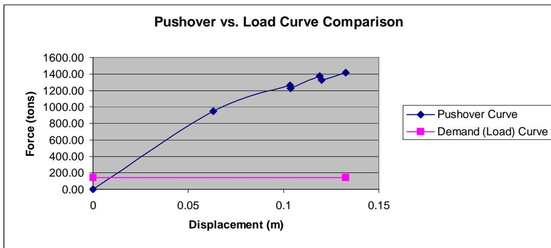
**Figure 50:** Pushover curve and Load curve comparison for the determination of Progressive Collapse two column removal in the long side of the building.
