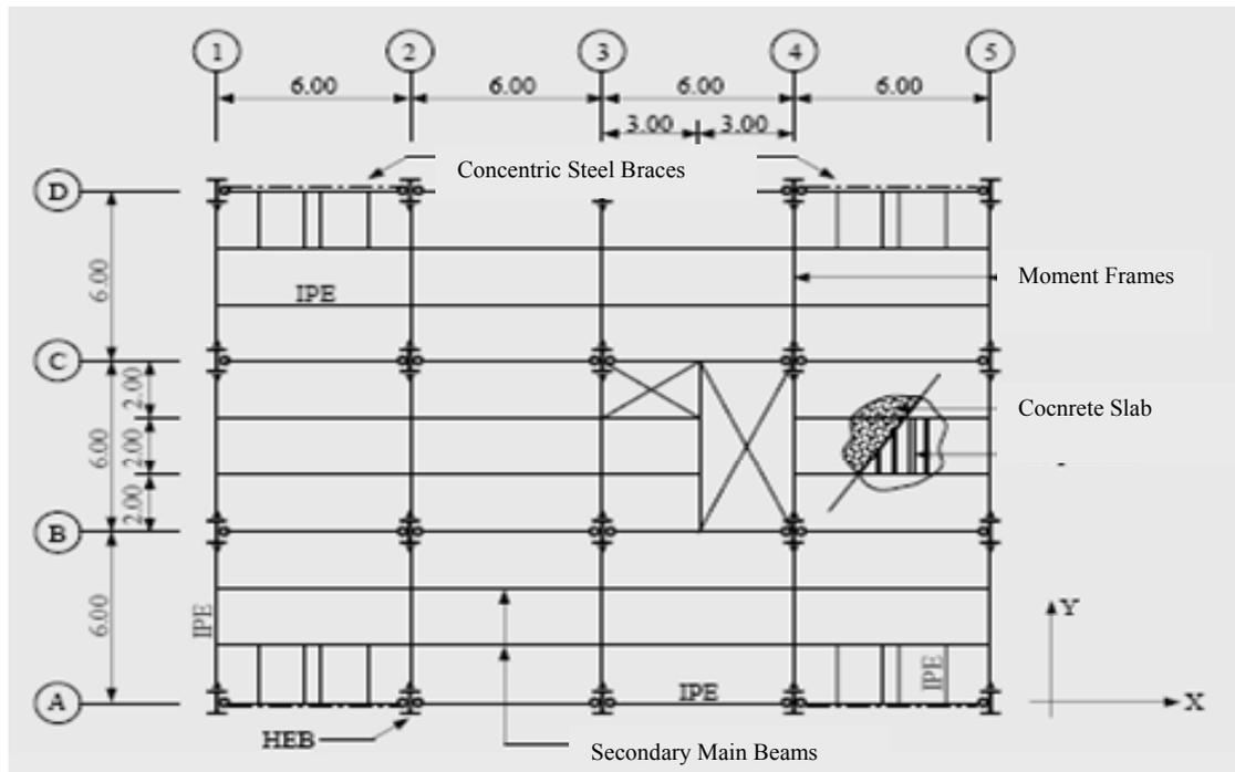
**Figure 34:** Story plan of six story model steel building.
