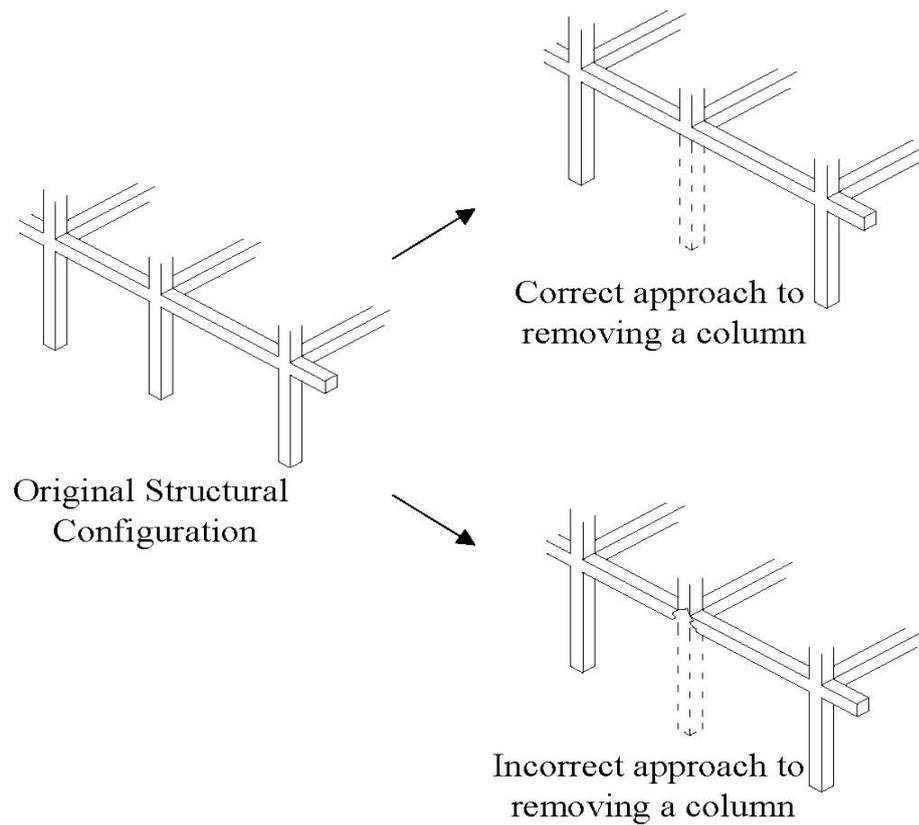
**Figure 24:** Sketch of the correct and incorrect approach for removing a column.
