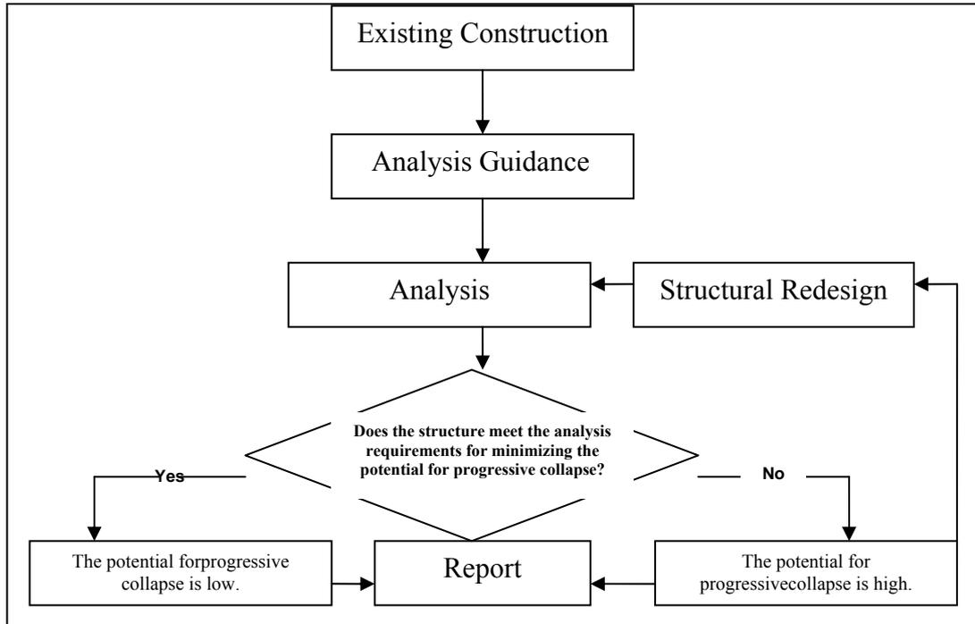
**Figure 19:** Process for reducing the potential for progressive collapse in new construction. (based on PCADG of GSA, 2003)
