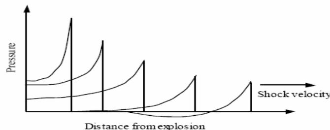
**Figure 2:** Blast Wave Propagation.
