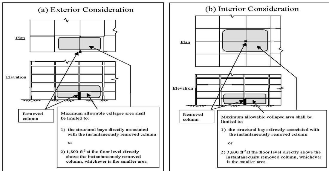
**Figure 20:** : An example of maximum allowable collapse areas for a structure that uses columns for the primary vertical support system. (from PCADG of GSA, 2003)
