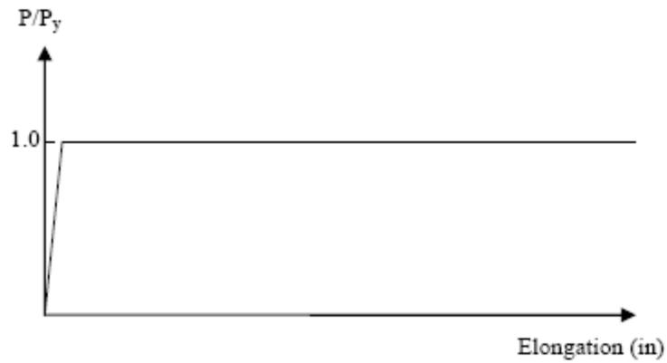
**Figure 28:** Axial Hinge Properties.
