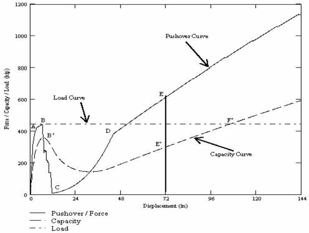
**Figure 30:** Pushover Curve, Capacity Curve, and Load Curve.
