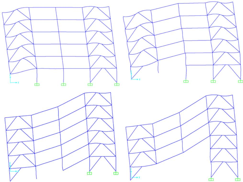
**Figure 48:** Step by Step Progressive Collapse initiation of the model building.
