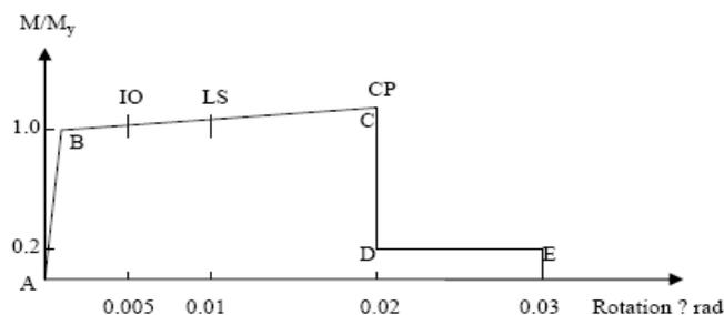
**Figure 27:** Moment Hinge Properties.(from work of Gilsanz and Guo, 2003)
