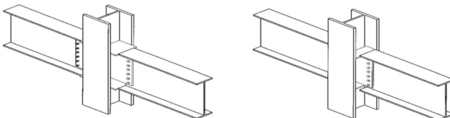
**Figure 23:** (a) Fully Rigid Connection (b) Typical Shear Only Connection
