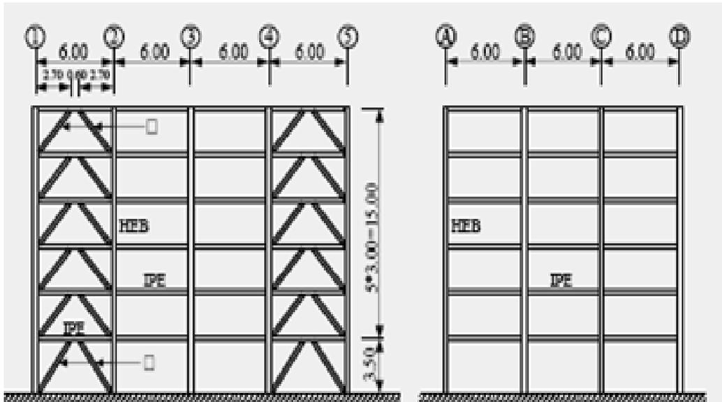
**Figure 35:** Framing system of the building in perpendicular directions.
