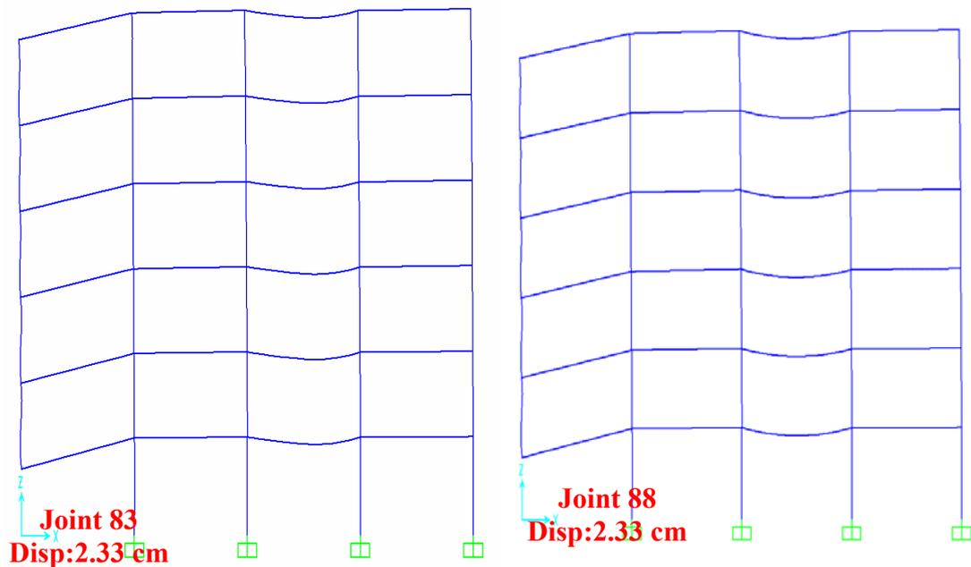
**Figure 47:** Deformed shape and maximum deformation of the framing system after two column removal in short direction. (cross-section of the frame)
