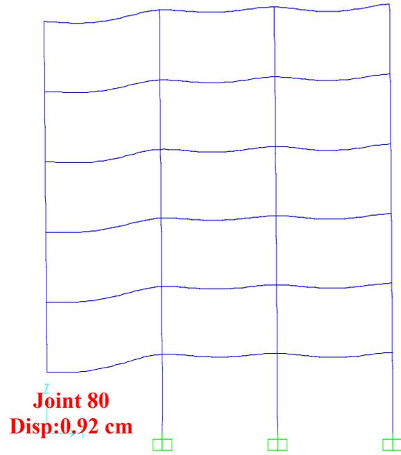
**Figure 41:** Cross section of the frame Deformed shape and maximum deformation of the framing system after one column removal in long direction per GSA, PCADG.
