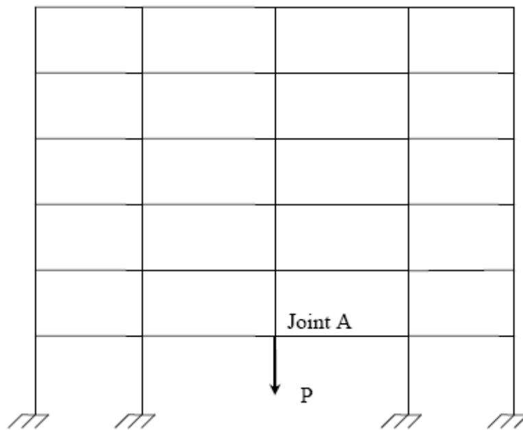
**Figure 29:** Loading for Pushover Analysis Procedure.
