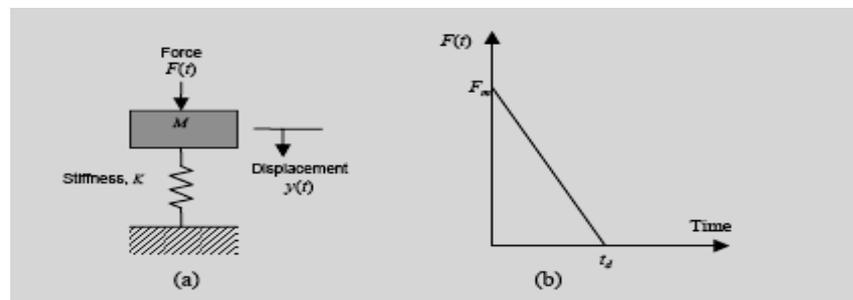
**Figure 9:** (a) SDOF system and (b) blast loading.
