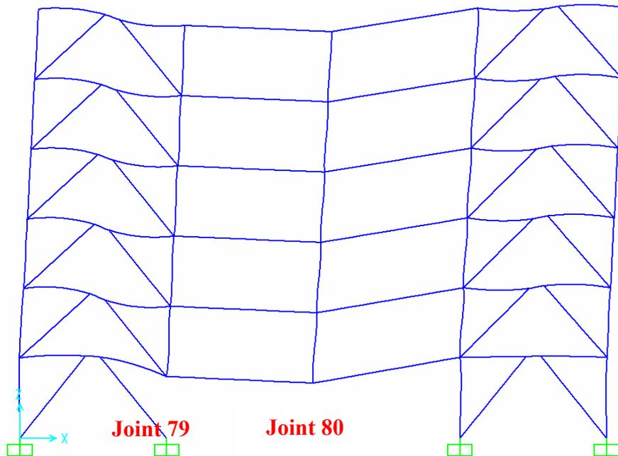
**Figure 42:** Deformed shape of the framing system after two column removal in long direction.
