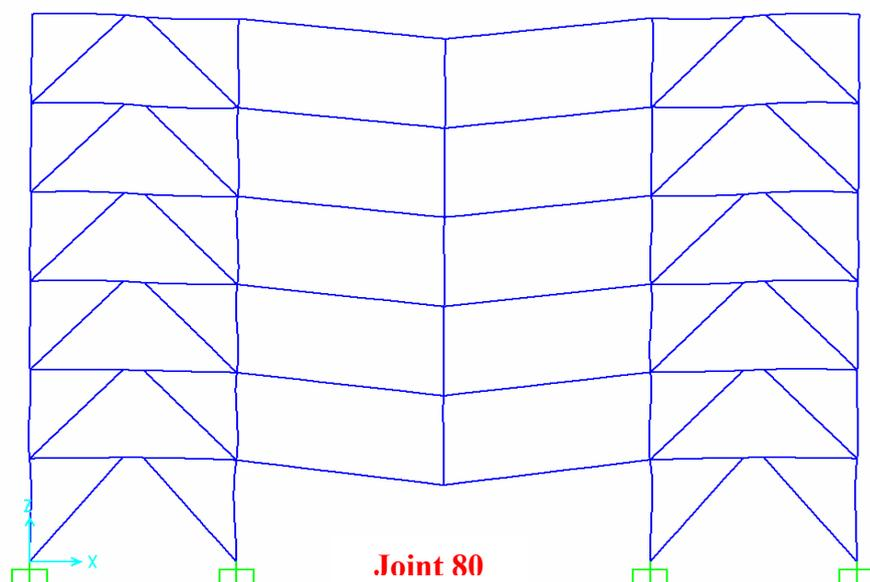
**Figure 40:** Deformed shape of the framing system after one column removal in long direction per GSA, PCADG.
