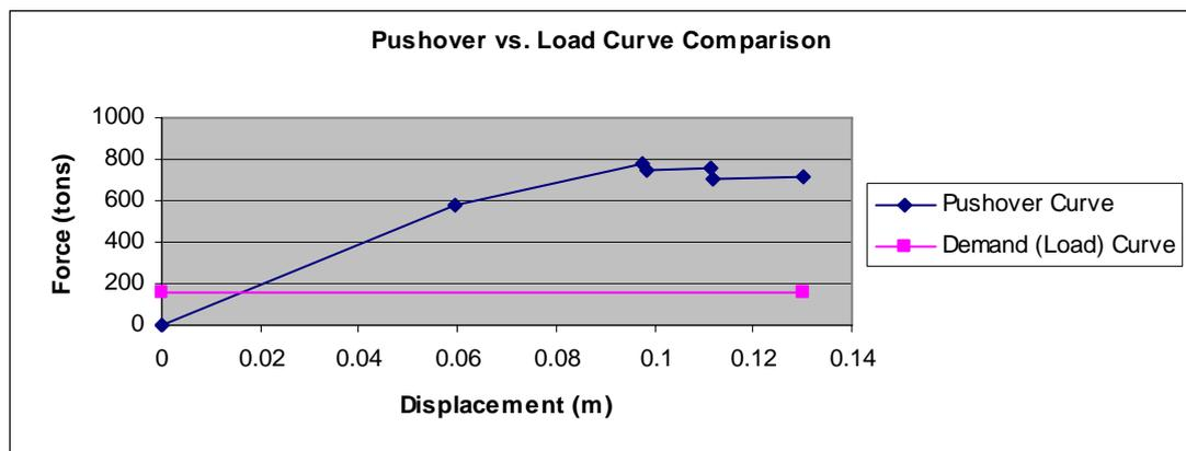
**Figure 52:** Pushover curve and Load curve comparison for the determination of Progressive Collapse two column removal in the short side of the building.
