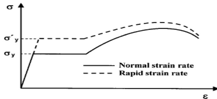
**Figure 8:** Strain rate effect on structural steel.
