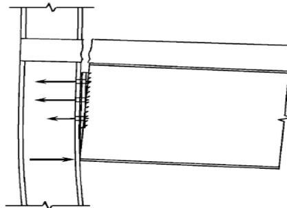
**Figure 15:** Prying action at steel connections.
