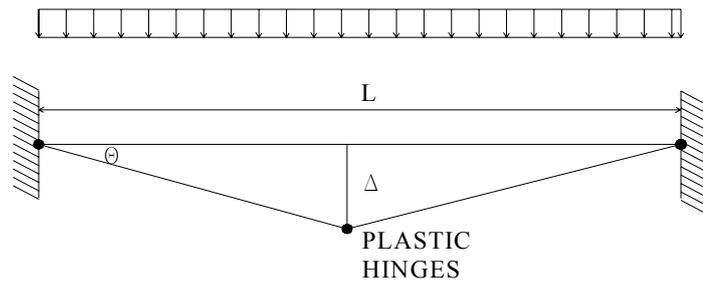
**Figure 21:** Formation of Failure Mechanism.
