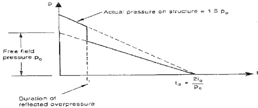
**Figure 5:** Transient Pressure at the center of the target.
