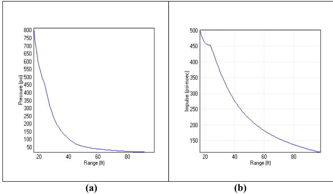
**Figure 37:** (a) Pressure and (b) impulse diagrams of explosion of 500 kg ANFO.
