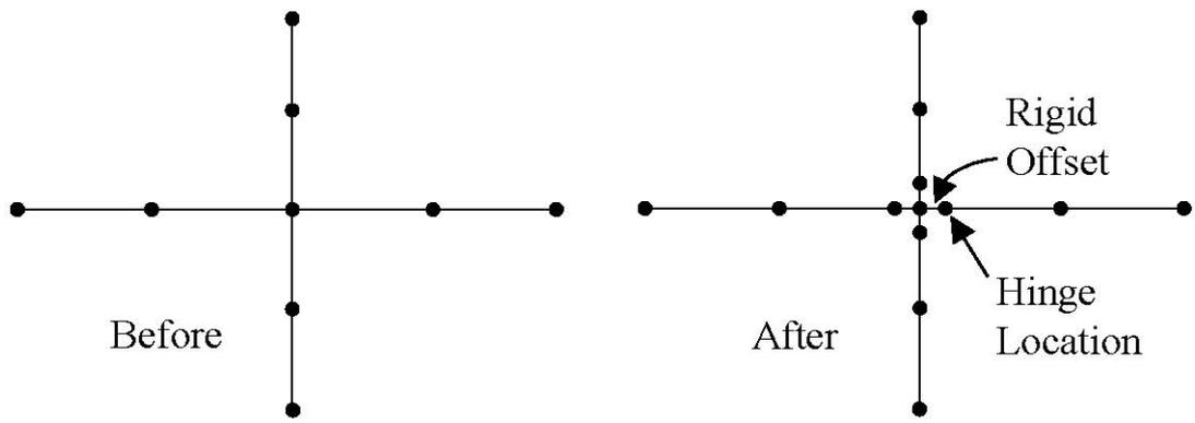
**Figure 22:** Rigid offset placement.
