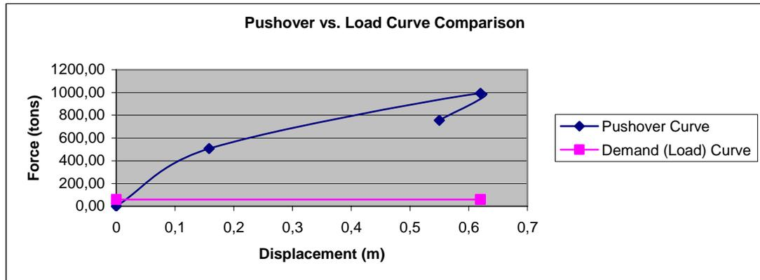
**Figure 49:** Pushover curve and Load curve comparison for the determination of Progressive Collapse for one column removal.in the long side.
