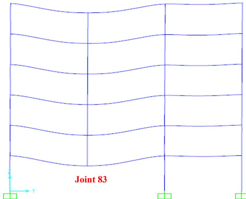
**Figure 44:** Deformed shape of the framing system after one column removal in short direction.
