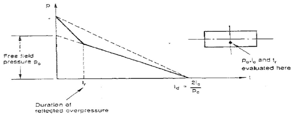
**Figure 6:** Transient Pulse at the center of the target.
