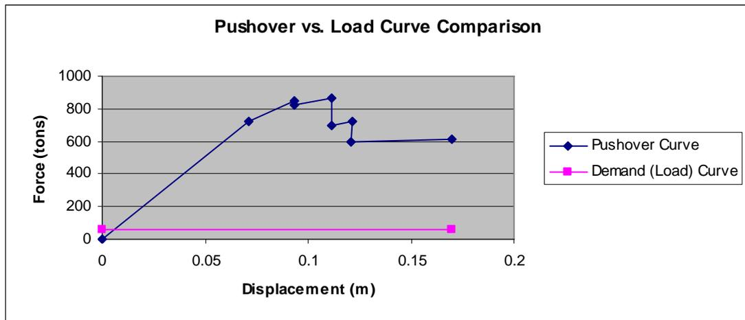
**Figure 51:** Pushover curve and Load curve comparison for the determination of Progressive Collapse for one column removal in the short side of the building.
