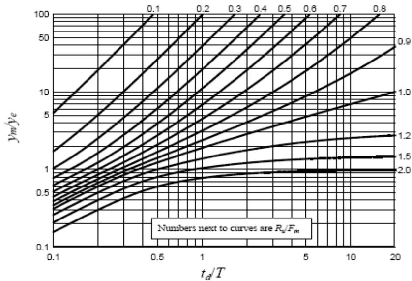
**Figure 11:** Maximum response of elastoplastic SDF system to a triangular load.
