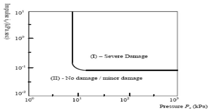
**Figure 14:** Typical Pressure-impulse (P-I) diagram.
