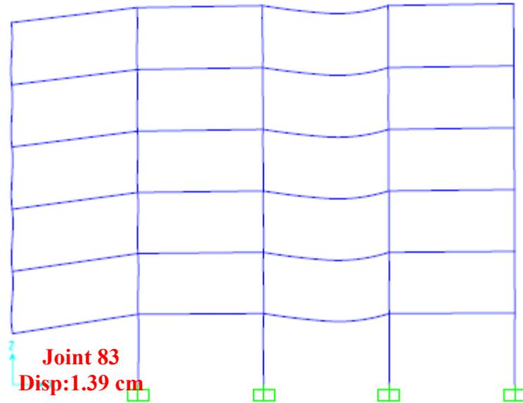
**Figure 45:** Deformed shape and maximum deformation of the framing system after one column removal in short direction. (cross-section of the frame)
