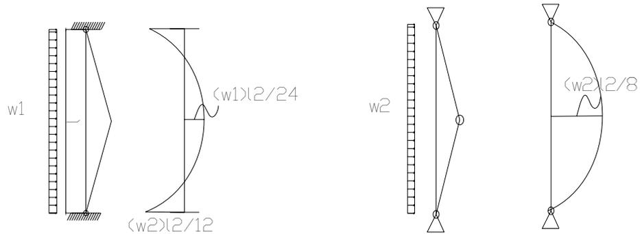
**Figure 38:** Formation of Three Hinge mechanism under bending moment action.
