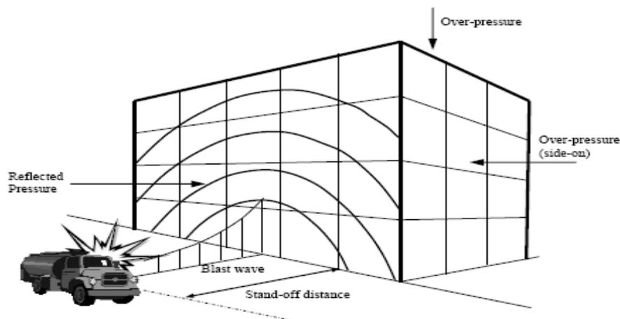
**Figure 3:** Blast loading on a building.
