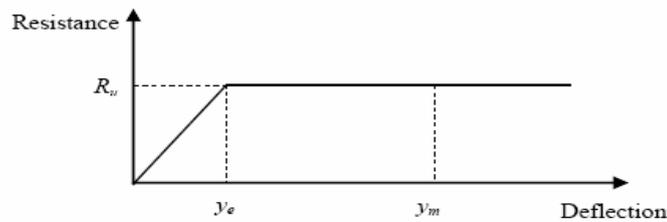
**Figure 10:** Simplified resistance function of an elastoplastic SDOF system.
