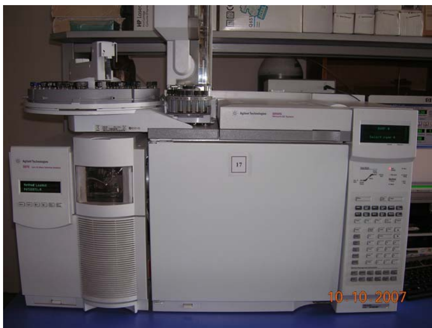
Figure 2.1 The GC-MS System used in the study.
