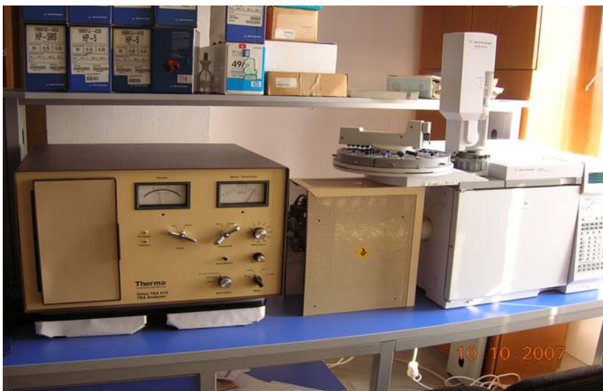
Figure 2.2 The GC-TEA System used in the study.
