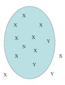
*Figure 2.3: N is a new case. It would be assigned to the class X because the seven X's within the ellipse outnumber the two Y's (cf. also [158]).*
