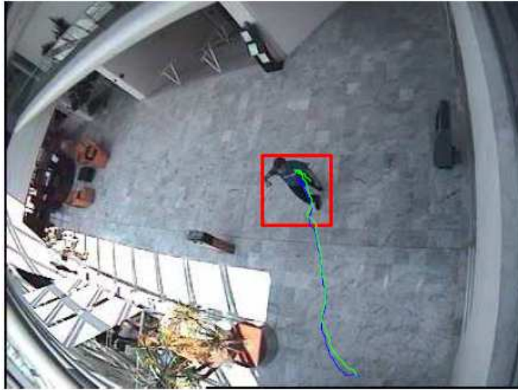
Figure 4.2 Kalman Tracker: Estimated and real trajectories of a moving object
