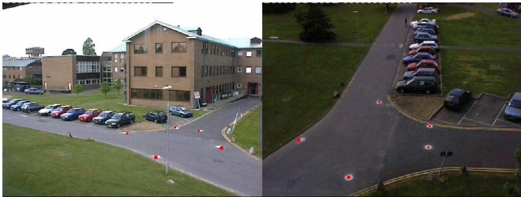
Figure 5.2 Point transfer by using homography matrix
