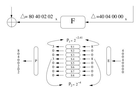
Figure 2.4: A One Round Differential for DES
