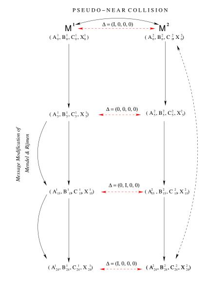
Figure 4.4: Pseudo-Near-Collision Attack on Tiger
