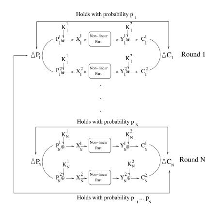
Figure 2.3: Overview of the Differential Cryptanalysis
