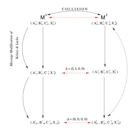
Figure 4.3: Collision Attack on Tiger-16
