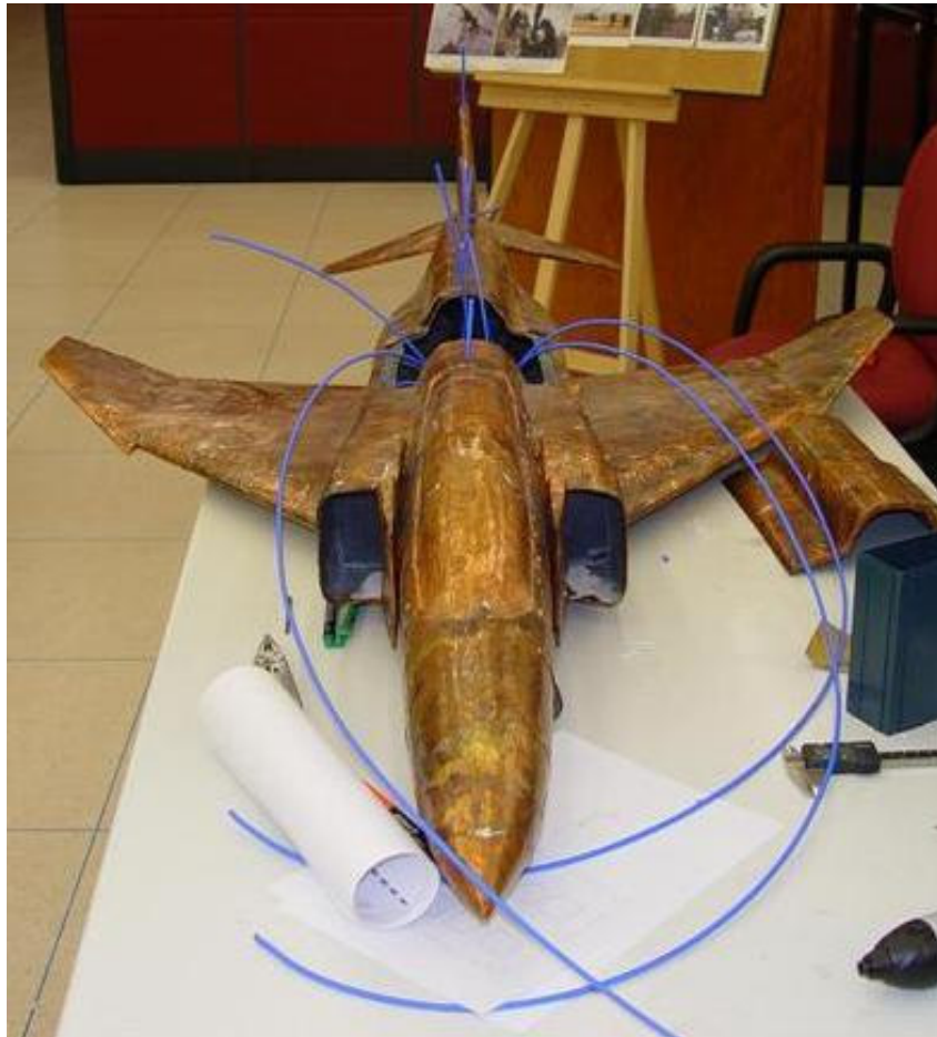
Figure 4-1 Overall view of model cabling (top cover removed)
