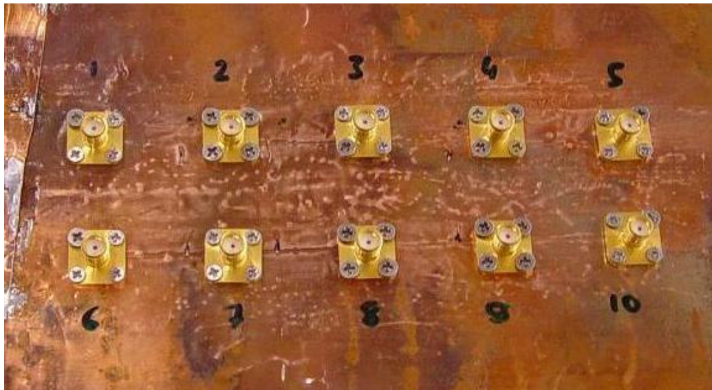
Figure 4-3 SMA (female) connectors assembled on bottom face
