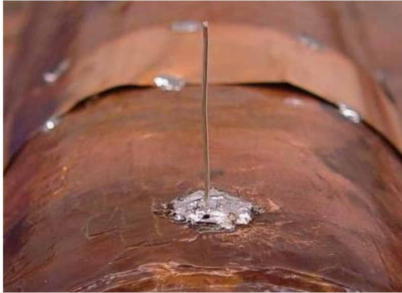
Figure 4-4 Detailed view of a monopole over the fuselage
