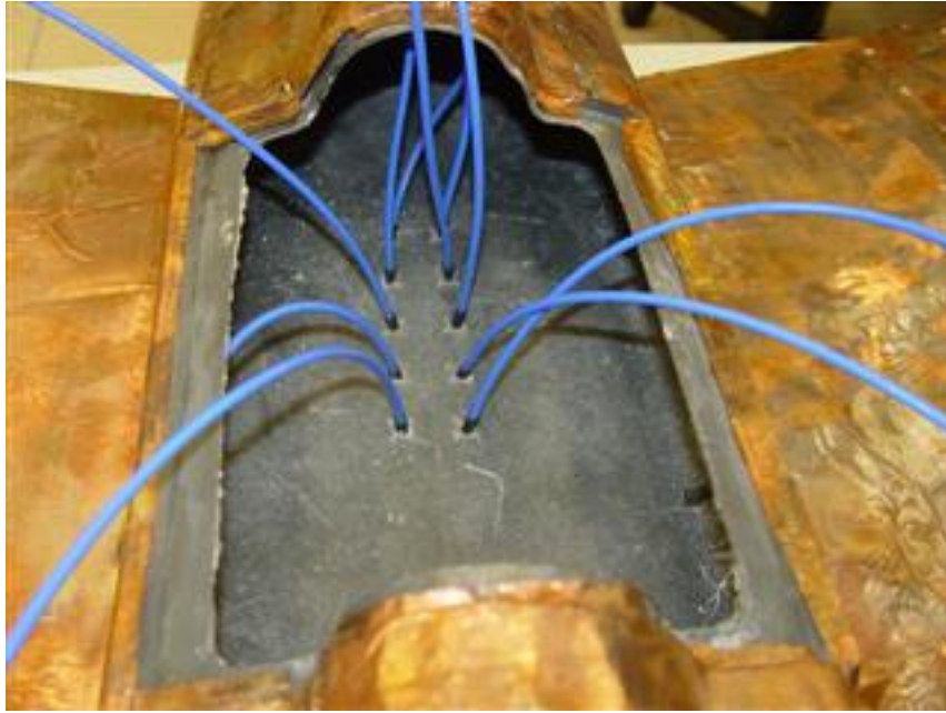
Figure 4-2 Detailed view of coaxial cables inside the fuselage (top cover opened)
