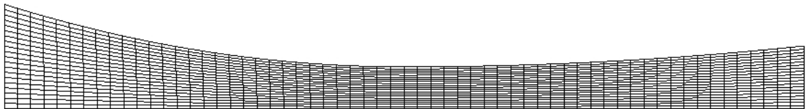
Figure 3.15: 61x21 mesh used in 2D Converging-Diverging Half Nozzle problem
