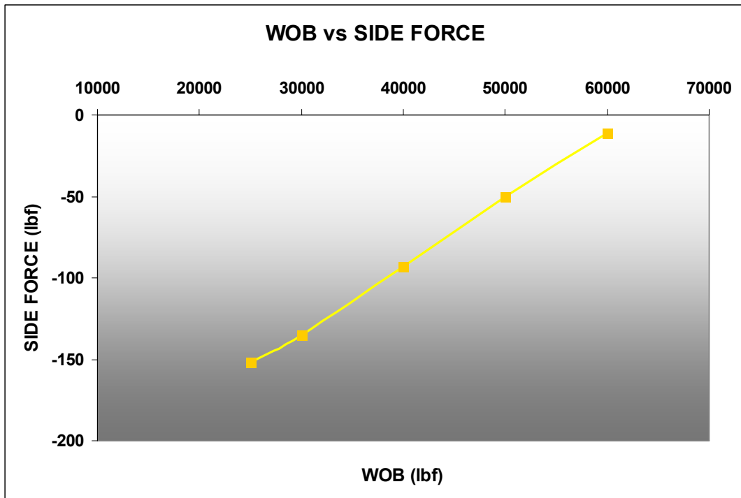
Fig.19 WOB vs Side Force for Slick Assembly
