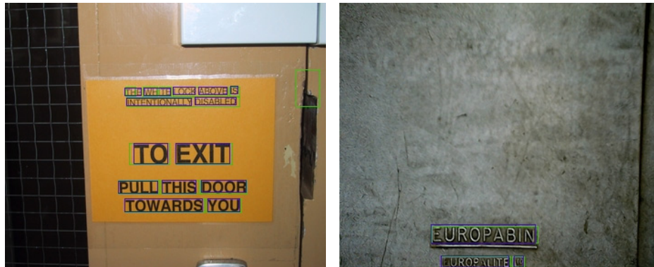
Figure 26: Localization results (Green boxes indicate results due to the proposed algorithm whereas blue rectangles are the ground-truth).
