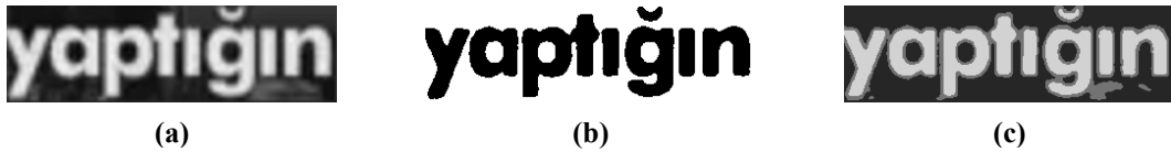
Figure 19: (a) Source image; (b) Thresholding result by Kapur; (c) k-Means based segmentation result with 3 clusters. Characters p and t emerge as touching characters
