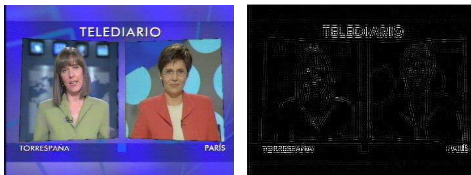
Figure 4: Example capture frame and reconstruction of the frame from selected DCT coefficients.
