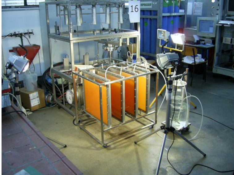
Figure 5.4. Four 5L photobioreactors connected in parallel (illuminated by 3x500W halogen lamps, frames of bioreactors are made of PVC, panels are from acrylic, the plates were inserted in a metal support).
