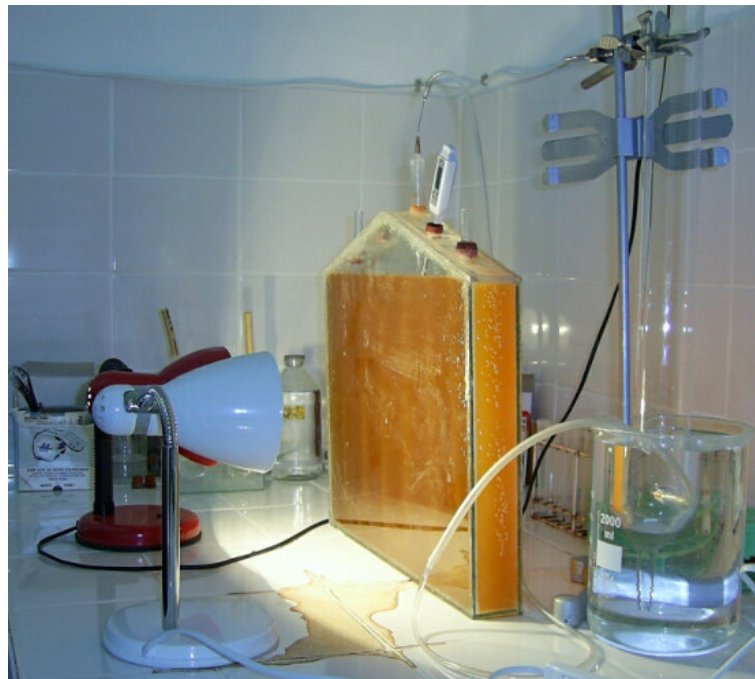
Figure 5.3. 5.5L photobioreactor (illuminated by 2x75W tungsten lamps, bioreactor made of glass and acrylic (top part only)).
