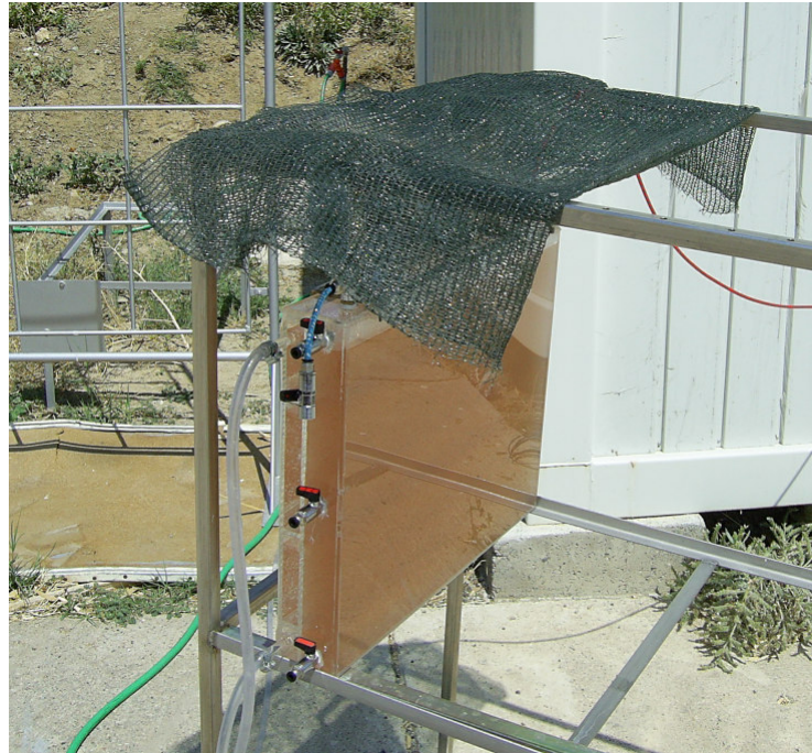
Figure 5.1. 8L acrylic photobioreactor (illuminated by sunlight).
