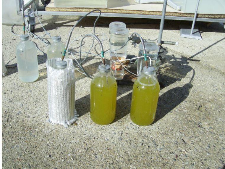
Figure 5.2. 0.5L glass photobioreactors (illuminated by sunlight).
