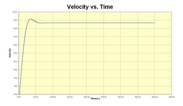
Figure 5.7: NSTMSS turning circle velocity change
