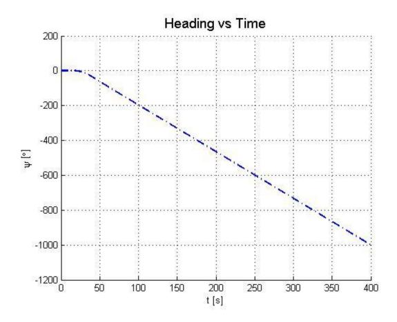
Figure 5.6: Matlab turning circle heading angle change
