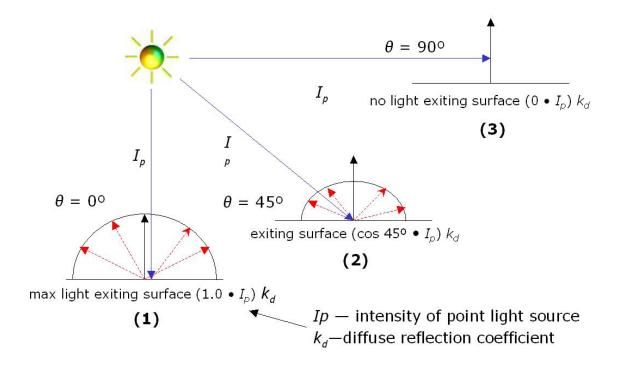
Figure 3.15: Diffuse reflection according to the angles
