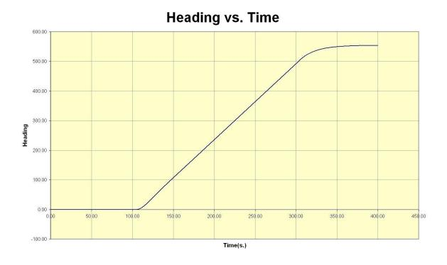
Figure 5.15: NSTMSS pull out heading change
