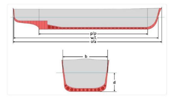
Figure 4.2: Main geometric features of a ship
