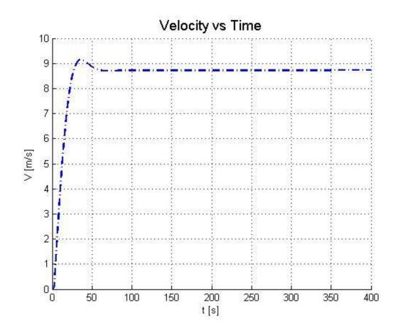
Figure 5.8: Matlab turning circle velocity change
