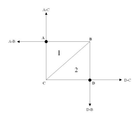
Figure 3.21: Normal Vectors and Quad Mesh Relation
