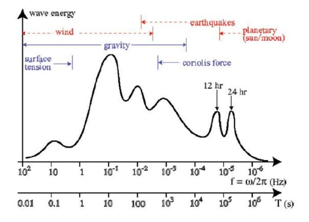
Figure 3.4: Wave Energy Spectra of Ocean Waves
