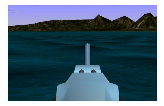
Figure 3.11: Appearance of the ship waves with normal mesh method
