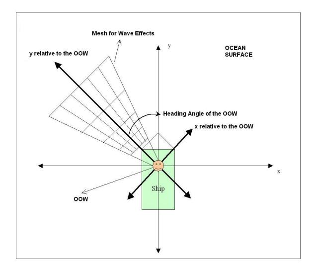
Figure 3.10: Adaptive mesh position according to the OOW
