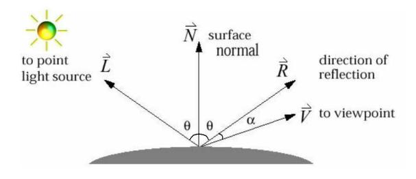
Figure 3.17: Specular reflection according to the angles
