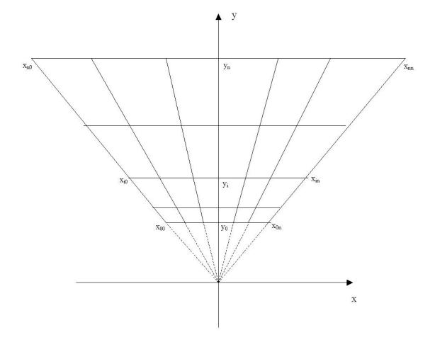
Figure 3.9: Adaptive surface mesh generation top view
