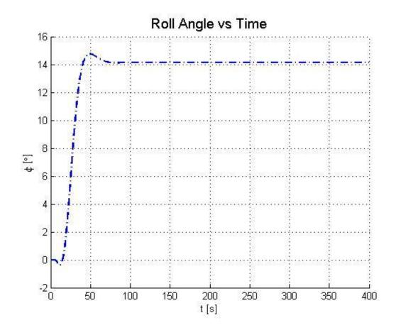
Figure 5.2: Matlab turning circle roll angle change
