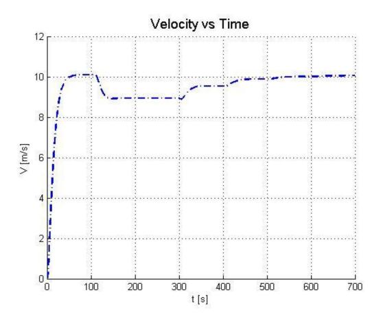
Figure 5.26: Matlab spiral maneuver velocity change
