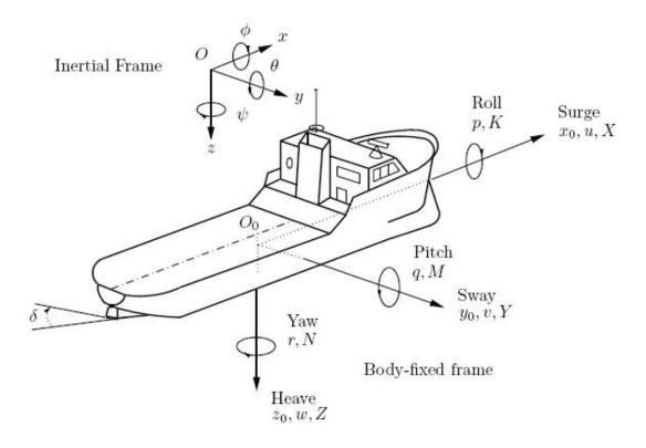
Figure 4.1: Reference Frames and Motion Variables
