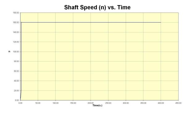
Figure 5.9: NSTMSS turning circle shaft speed change
