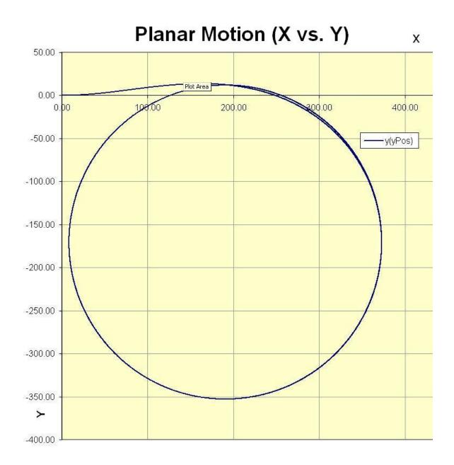
Figure 5.3: NSTMSS turning circle planar motion change
