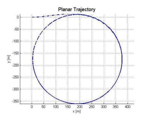
Figure 5.4: Matlab turning circle planar motion change
