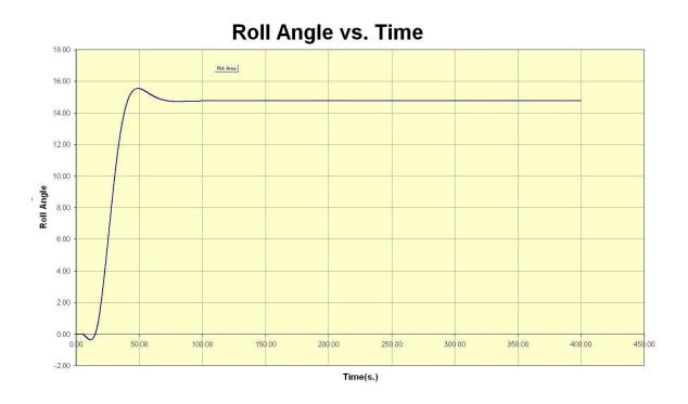
Figure 5.1: NSTMSS turning circle roll angle change
