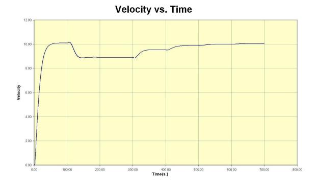
Figure 5.25: NSTMSS spiral maneuver velocity change
