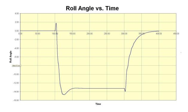
Figure 5.19: NSTMSS pull out roll change
