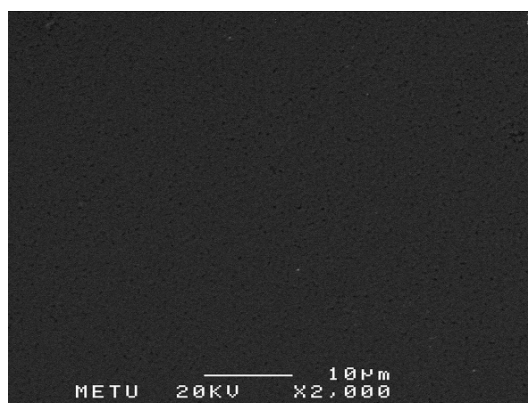
Figure 4.31 SEM image of the surface of PNZT thin film with composition \text{Pb}_{0.985}(\text{Zr}_{0.53}\text{Ti}_{0.47})_{0.97}\text{Nb}_{0.03}\text{O}_3 and sintered at 600 °C for 3 h.
