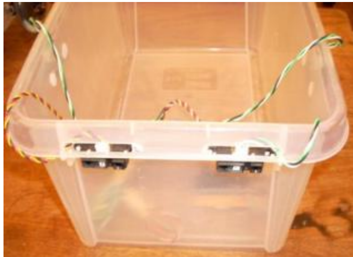
Figure 14: Infrared Range Sensor Module Prototype
