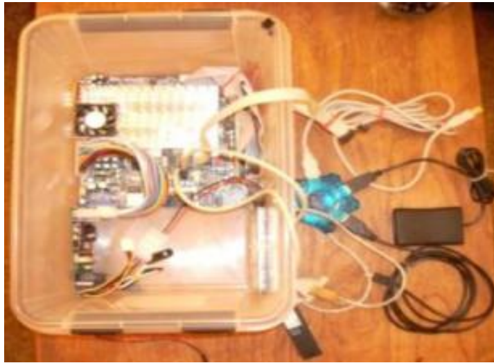
Figure 13: Main Controller Module Prototype
