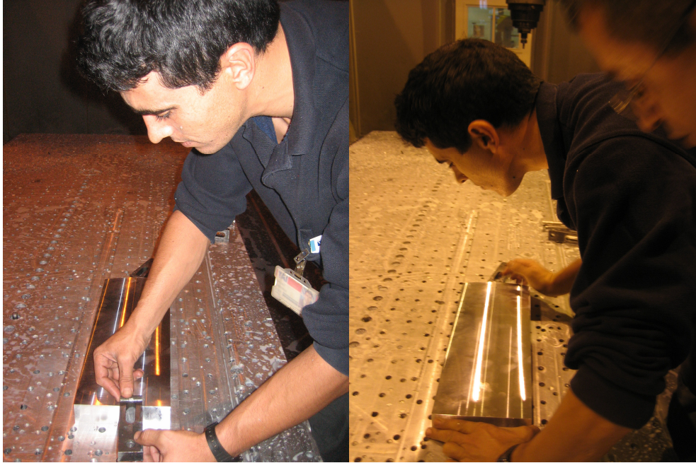
Figure 5.9 and Figure 5.10 Clamping of the material to the manufacturing board.
