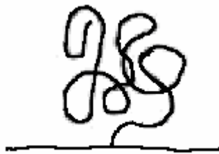
Figure 1.7 “Mushroom-like” conformation type of PEG side chains [17]
