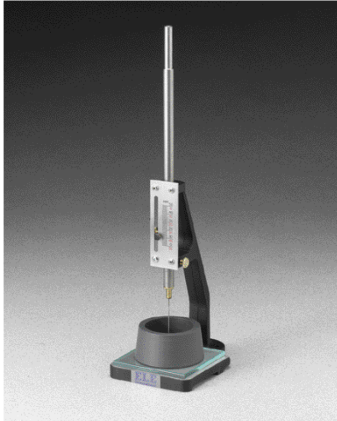
Figure 1.9 Vicat apparatus for setting time test *
