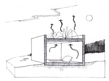
Figure 2.16 Roof sprinkling systems for cooling Source: Heerwagen, 2004, p. 156
