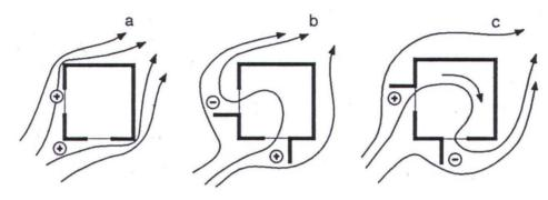
Figure 2.05 Basic air flow principles, (iv) Source: Goulding, 1994, p. 103
