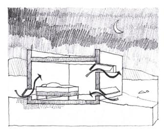
Figure 2.09 Nocturnal ventilative cooling Source: Heerwagen, 2004, p. 151
