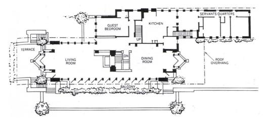
Figure 2.08 An example for comfort ventilation, Robie House in Chicago Source: Lechner, 1991, p.197
