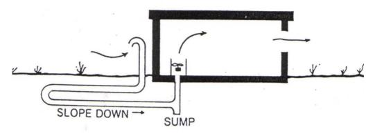
Figure 2.18 Indirect earth cooling system with pipes Source: Lechner, 1991; p.205
