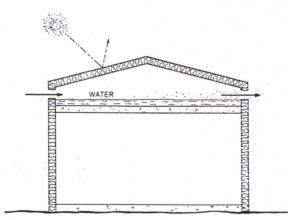
Figure 2.14 Roof pond system with fixed insulation Source: Lechner, 1991, p. 201
