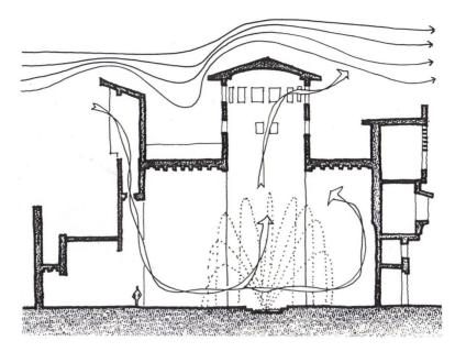
Figure 2.12 Direct evaporative cooling with the use of an interior fountain Source: Moore, 1993
