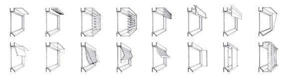
Figure 2.01 External shading devices Source: Goulding, 1994, p. 102
