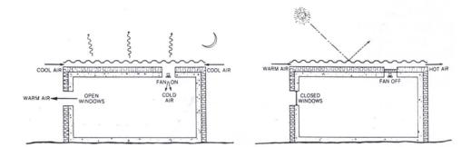
Figure 2.11 Indirect radiative cooling system Source: Lechner, 1991, p.200
