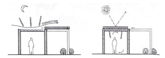
Figure 2.10 Direct radiative cooling system Source: Lechner, 1991, p.200
