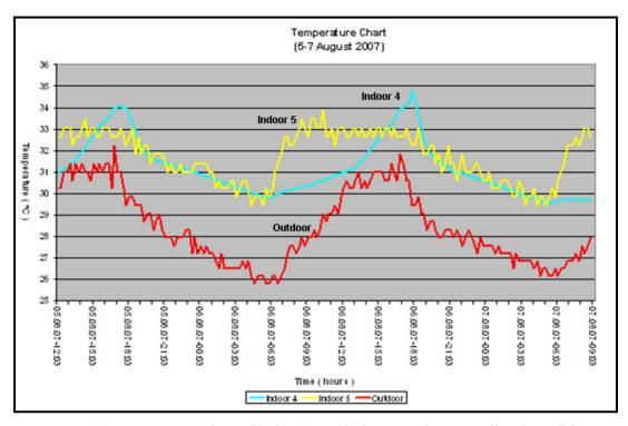
Figure 4.05 Temperature chart of indoor 4 and indoor 5 under unventilated conditions
