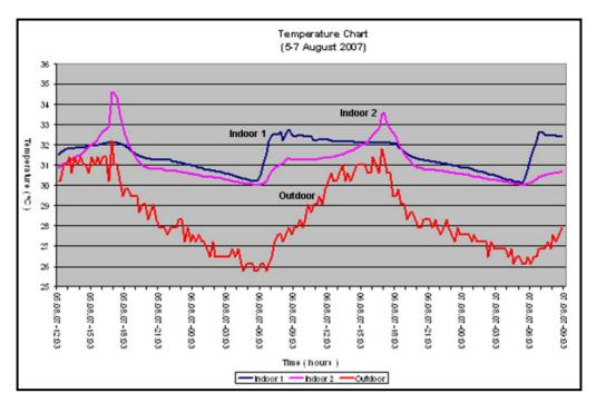
Figure 4.06 Temperature chart of indoor 1 and indoor 2 under unventilated conditions
