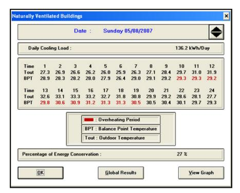
Figure 4.10 Hourly balance point temperatures under natural ventilation (5 August 2007)
