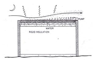
Figure 2.15 Roof pond system with floating insulation Source: Givoni, 1994, p. 152
