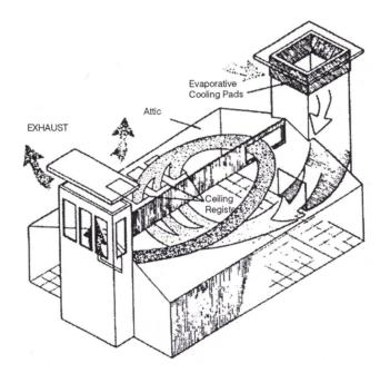
**Figure 2.13** Evaporative cooling towers Source: Santamouris and Assimakopoulos, 1996, p. 409
