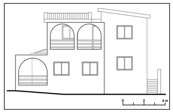
Figure A.03 East elevation of case study building
