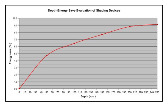
Figure 4.11 Depth vs. energy savings chart of shading devices
