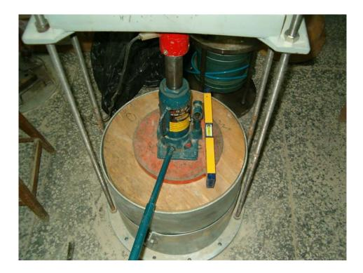
Figure 4.2 Compressing of the soil layers
