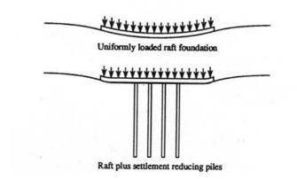
Figure 2.3 Central piles to reduce differential settlement (Randolph, 1994)
