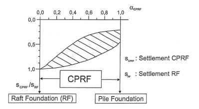
Figure 2.2 Foundation settlements as a function of piled raft coefficient (Katzenbach et al., 2005)
