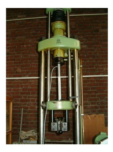
Figure 4.5 Calibration of a model pile in the mechanical press
