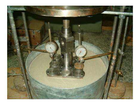
Figure 5.2 Plain raft test setup
