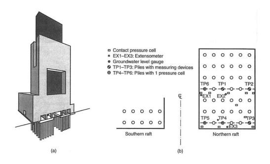
Figure 2.10 Messe-Torhaus building: a) isometric view,b) plan of piled raft with measuring devices (Franke et al., 2000)
