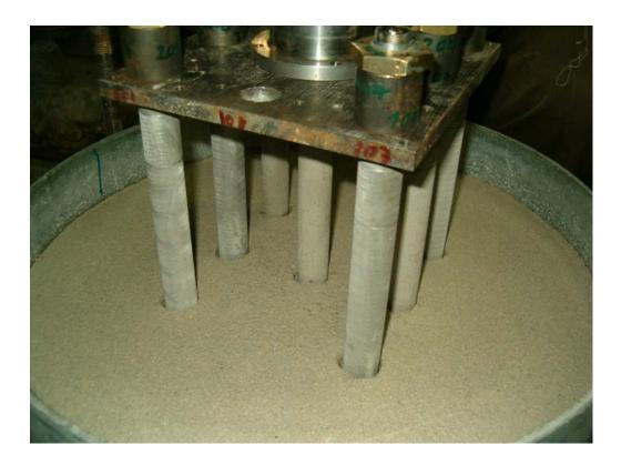
Figure 5.18 Model piled raft with 7 piles
