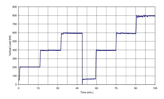
again with 400, 600 and 800 kN. At each increment load was kept constant for 15 minutes.
