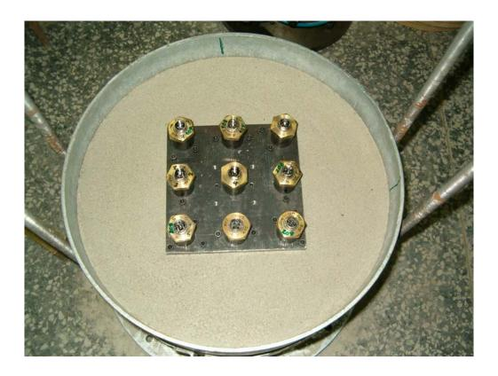
Figure 5.25 Model piled raft with 9 piles
