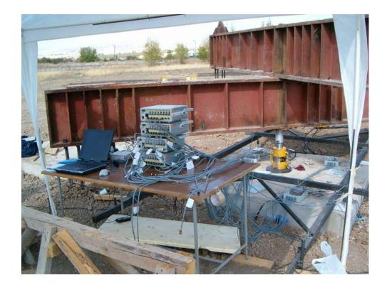
Figure 3.5 Loading and measurement systems
