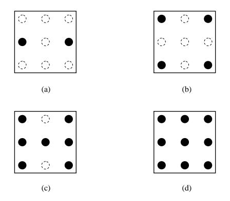
Figure 5.1 Model piled raft configurations: a) piled raft with 2 piles, b) piled raft with 4 piles, c) piled raft with 7 piles, d) piled raft with 9 piles
