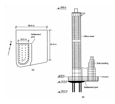
Figure 2.12 DG-Bank building: a) ground plan, b) sectional elevation (Katzenbach et al., 2000)
