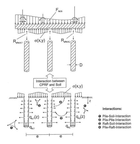
Figure 2.1 Soil-structure interaction of piled rafts (Katzenbach et al., 2004)
