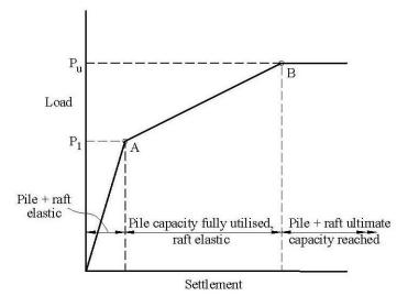
Figure 2.6 Simplified load-settlement curve (Poulos, 2000a, 2001)
