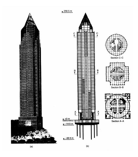
Figure 2.11 Messeturm building: a) elevation, b) cross-sections (Katzenbach et al., 2000)
