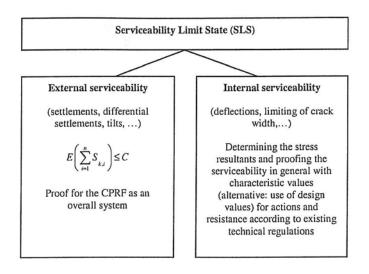
Figure 2.9 Serviceability Limit State (SLS) approach (Katzenbach et al., 2005)
