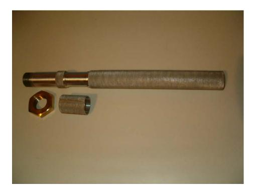
Figure 4.4 Model pile, cover plate and fixing element
