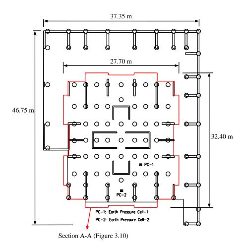
Figure 3.9 Plan view of the piled raft foundation of the building
