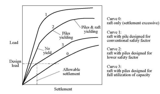
Figure 2.4 Load-settlement curves for piled rafts according to various design philosophies (Poulos, 2000a)
