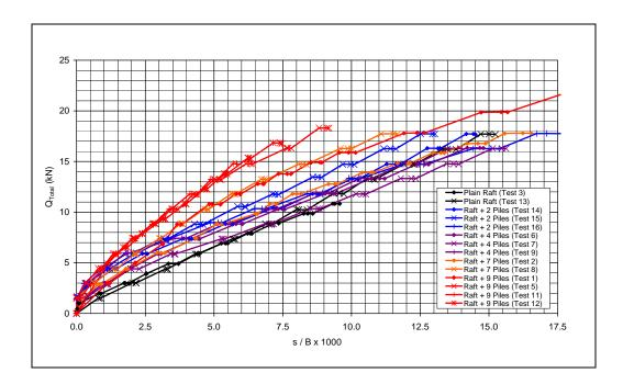
Figure 6.12 Load – settlement relationships of piled rafts and plain raft
