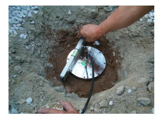
Figure 3.12 Placing and leveling of the earth pressure cell
