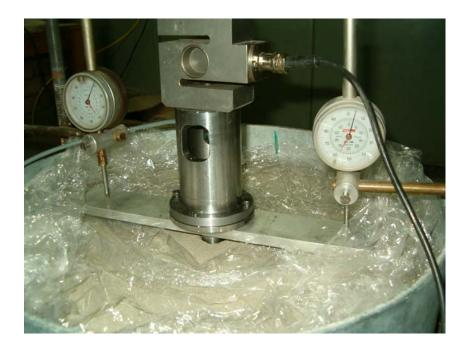
Figure 5.5 Single pile test setup
