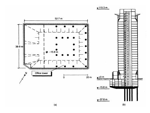
Figure 2.13 Japan-Centre building: a) ground plan b) sectional elevation (Katzenbach et al., 2005)
