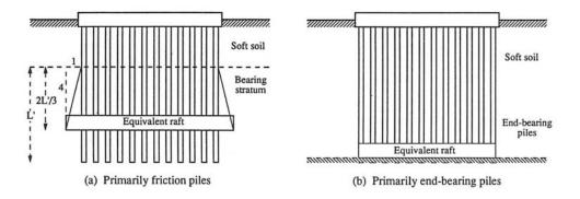
Figure 2.5 Equivalent raft approach for pile groups (Randolph, 1994)
